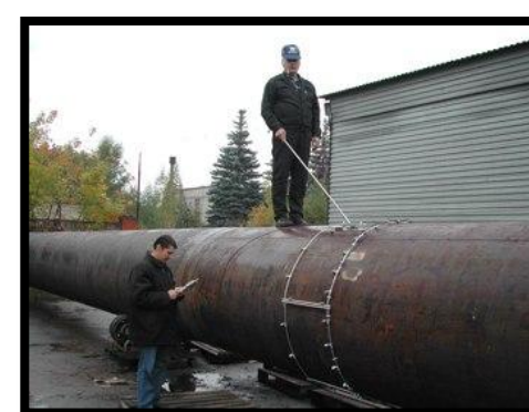
Remote non-destructive control (acoustic and magnetic tomography)
