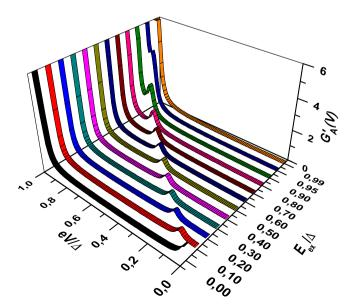
**Fig. 2.** The bias voltage dependence of differential conductance at zero temperature for exchange fields,  $E_{\rm ex}/\Delta=0$ , 0.1, 0.2, 0.3, 0.4, 0.5, 0.6, 0.7, 0.8, 0.9, 0.95 and 0.99. Here  $G_A'=2R_TG_A$ , W=0.014 and  $d_f=10\xi_{\rm s}$ .
