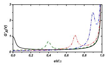
**Fig. 1.** The bias voltage dependence of differential conductance at zero temperature for exchange fields,  $E_{\rm ex}/\Delta=0$  (black solid line),  $E_{\rm ex}/\Delta=0.4$  (green dashed line),  $E_{\rm ex}/\Delta=0.7$  (red dash-dot-dotted line), and  $E_{\rm ex}/\Delta=0.9$  (blue dash-dotted line). Here  $G_A''=2R_TG_A$ , W=0.014 and  $d_f=10\xi_S$ . (For interpretation of the references to color in this figure caption, the reader is referred to the web version of this paper.)
