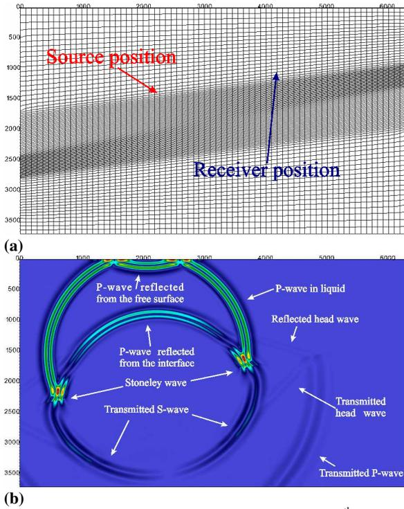
Figure 4: The grid used for the test #2 (every 10<sup>th</sup> line is plotted) (a); snapshots of the wave field (velocity modulus is plotted) at 1.3 sec (b)
