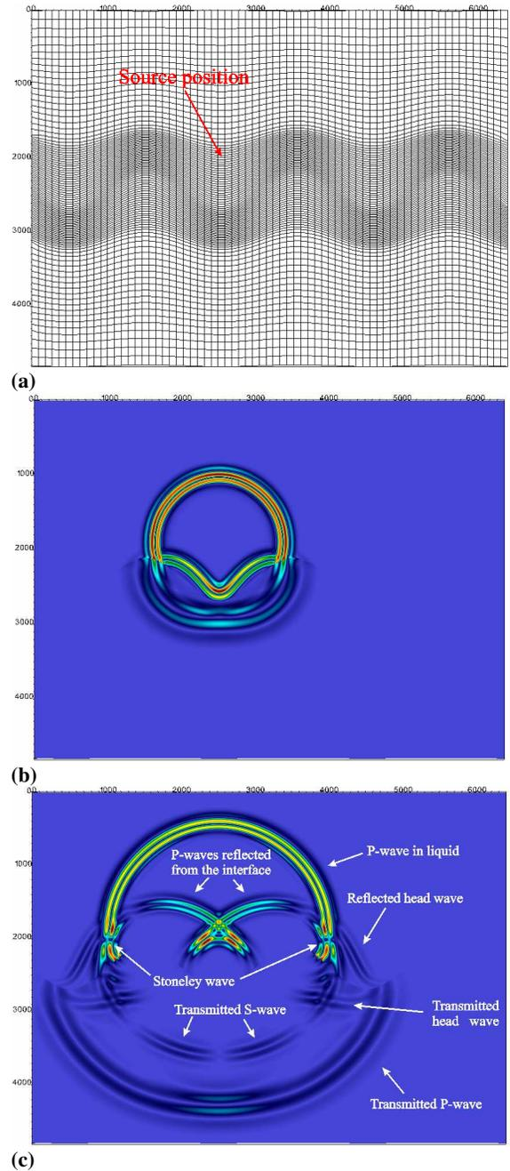
Figure 5: The grid used for the test #3 (every 10<sup>th</sup> line is plotted) (a); snapshots of the wave field (velocity modulus is plotted) at 0.8 sec (b) and 1.2 sec (c)
