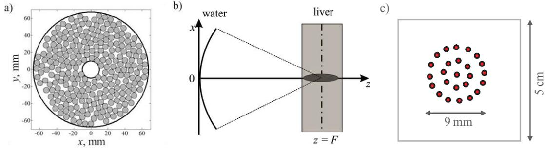
**FIGURE 1.** (a) Distribution of radiating elements on the surface of the therapeutic array; (b) geometry of the numerical experiment: ultrasound beam is focused within tissue layer (liver) centered at the geometric focus of the spherical shell ( $z = F$ ); (c) Discrete trajectory of the beam's focus in the focal plane. Acoustical modeling was done both in water and in liver sample, while temperature modeling was done only in liver.
