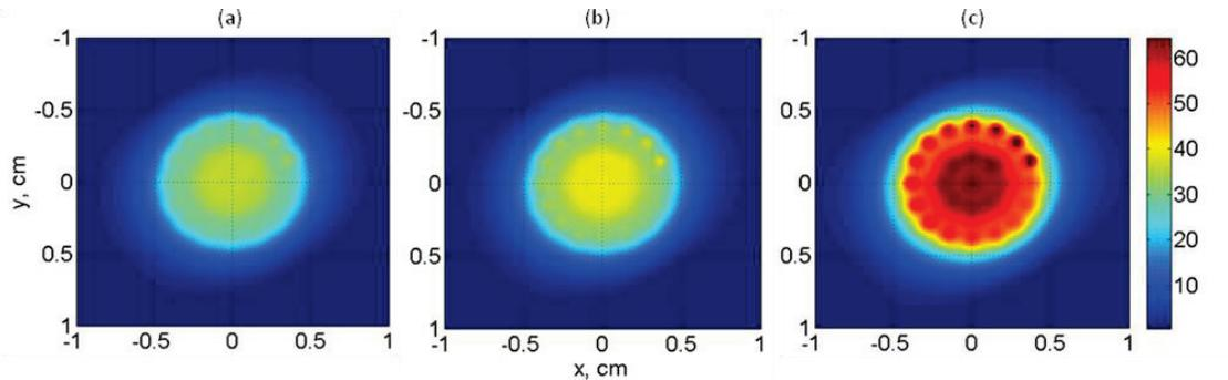
**FIGURE 4.** Temperature rise maps in the focal plane after 12 seconds of sonication for protocols with the same time-average power but different peak intensity at the array elements of  $1.2 \text{ W/cm}^2$  (a),  $4 \text{ W/cm}^2$  (b) and  $8 \text{ W/cm}^2$  (c).
