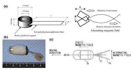
Fig. 5. (a) Magnetic swimming mechanism by use of alternating magnetic fields and a flexible tail by Sudo et al.<sup>128</sup> (b) Capsule with permanent magnet in a fin by Morita et al.<sup>132</sup> (c) Schematic from patent filing showing fish-like robot.<sup>135</sup> [Color figure can be viewed at wileyonline]
