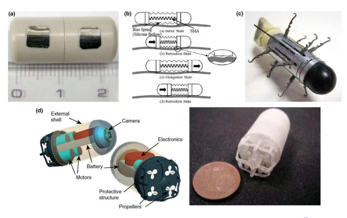
Fig. 2. Advanced WCE prototypes: (a) Capsule with patch electrodes for intestinal locomotion via electrically induced muscular contraction.<sup>33</sup> (b) SMA-based "Earthworm" capsule for intestinal locomotion.<sup>37</sup> (c) Twelve-legged capsule for crawling motion in the intestine,<sup>38</sup> (d) capsule with four propellers for swimming in a liquid-distended stomach.<sup>40</sup> [Color figure can be viewed at wileyonlinelibrary.com]
