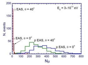
**Figure 4.** The distribution of EAS with primary energy  $E_0 = 3 \times 10^{13}$  eV produced by protons and  $\gamma$ -quanta (2) over the number of muons for zenith angles  $\theta = 0^\circ$  and  $\theta = 40^\circ$  at the altitude of observation.
