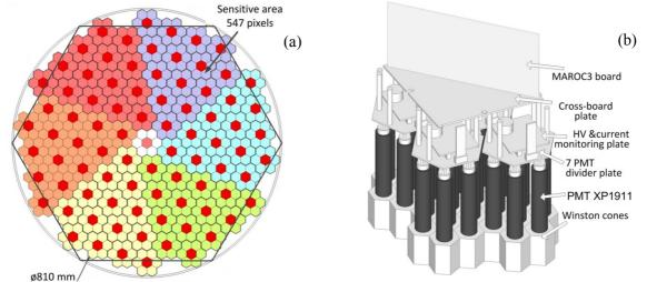
Figure 7. a) The matrix of pixels of the Tunka-IACT camera. b) The basic PMT block of TAIGA-IACT camera.
