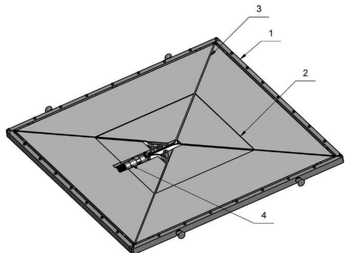
Fig. 3. The design of the muon detector: 1 – counter frame, 2 – scintillator, 3 – wavelength shifting bars, 4 – PMT. The size of the active surface is  $1 \times 1$  m<sup>2</sup>.
