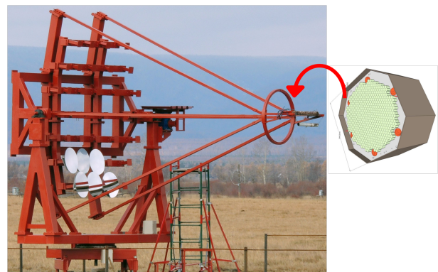
Figure 1. An IACT in the deployment phase (left panel) and a camera (right panel).
