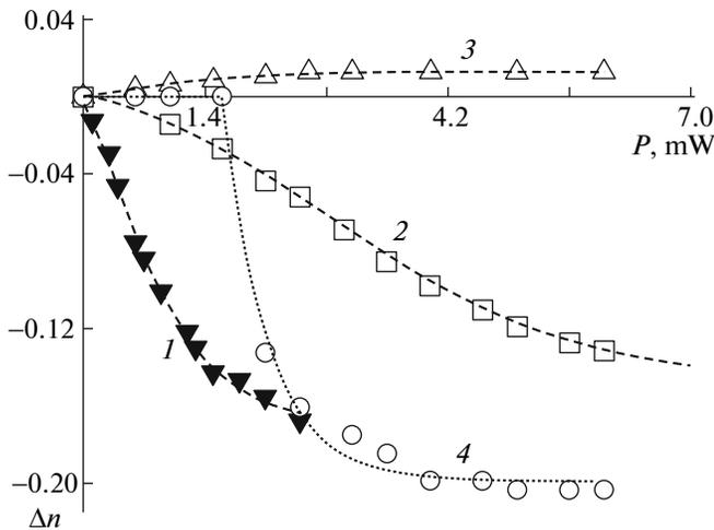
**Fig. 5.** Changes in refractive index  $\Delta n$  for an extraordinary wave plotted against light-beam power  $P$  ( $\lambda = 473$  nm) after light beam passage through planarly oriented ZhKM-1277 samples containing (1, 4) 0.5% polymer P-1, (2) 0.5% polymer P-2, and (3) 0.3% AD-1 dye. Curves 1–3 were obtained during oblique light wave incidence ( $\alpha = 50^\circ$ ); curve 4 was obtained under normal light incidence ( $\alpha = 0^\circ$ ).
