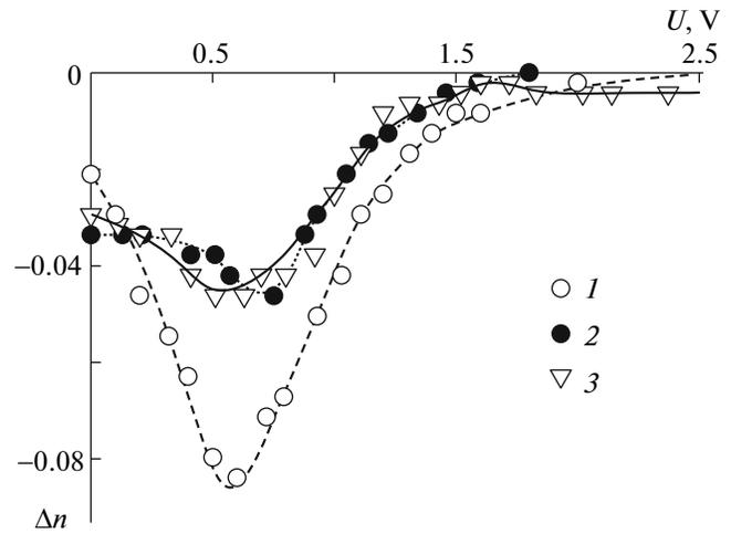
**Fig. 10.** Changes in refractive index  $\Delta n$  for the extraordinary wave plotted against low-frequency ( $\nu = 3$  kHz) voltage  $U$  for the planarly oriented samples: (1) ZhKM-1277 + 0.15% 2G dendrimer, (2) ZhKM-1277 + 0.15% 3G dendrimer, and (3) ZhKM-1277 + 0.15% 4G dendrimer:  $P =$  (1) 5, (2) 3, and (3) 2.6 mW.
