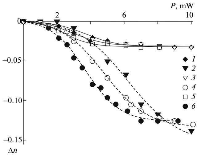
**Fig. 9.** Changes in refractive index  $\Delta n$  for the extraordinary wave plotted against light-beam power  $P$  ( $\lambda = 473$  nm) after light beam passage through (1, 3, 5) homeotropically and (2, 4, 6) planarly oriented ZhKM-1277 samples containing (1, 2) 0.15% 2G dendrimer, (3, 4) 0.15% 3G dendrimer, and (5, 6) 0.15% 4G dendrimer.
