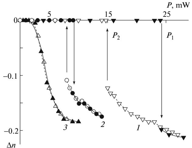
**Fig. 11.** Changes in refractive index  $\Delta n$  for the extraordinary wave plotted against light-beam power  $P$  ( $\lambda = 473$  nm,  $\alpha = 0^\circ$ ) after light beam passage through the planarly oriented samples based on ZhKM-1277 containing (1) 0.15% 2G dendrimer, (2) 0.15% 3G dendrimer, and (3) 0.15% 3G dendrimer: (closed symbols) increases and (open symbols) decreases in light-beam power  $P$ .
