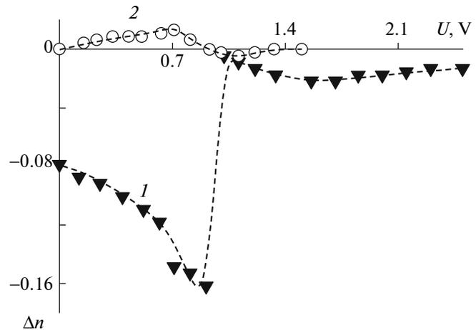
**Fig. 6.** Changes in refractive index  $\Delta n$  for an extraordinary wave ( $\lambda = 473$  nm,  $P = 1$  mW,  $\alpha = 40^\circ$ ) plotted against low-frequency ( $\nu = 3$  kHz) voltage  $U$  for the planarly oriented samples based on (1) ZhKM-1277 + 0.5% P-1 and (2) ZhKM-1277 + 0.3% AD-1.
