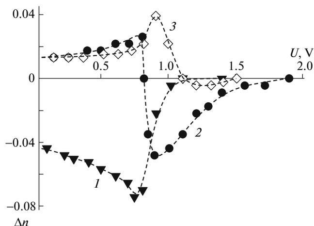
**Fig. 8.** Changes in refractive index  $\Delta n$  for the extraordinary wave ( $\lambda = 473$  nm,  $\alpha = 40^\circ$ ) plotted against low-frequency ( $\nu = 3$  kHz) voltage  $U$  for planarly oriented samples: (1) ZhKM-1277 + 0.1% 5G dendrimer, (2) ZhKM-1277 + 0.5% 1G dendrimer, and (3) ZhKM-1277 + 0.5% AD-2.
