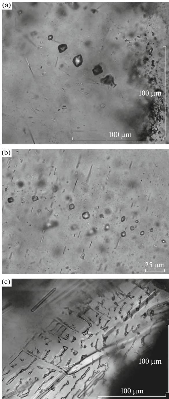
**Fig. 7.** CO<sub>2</sub> inclusions in granitoids from the Bandelierkop quarry (Safonov et al., 2018b). (a) Isolated group of quartz-hosted primary inclusions. (b) Chain of pseudo-secondary inclusions trapped along a crack in quartz. (c) Wedge-shaped pseudosecondary inclusions in quartz.
