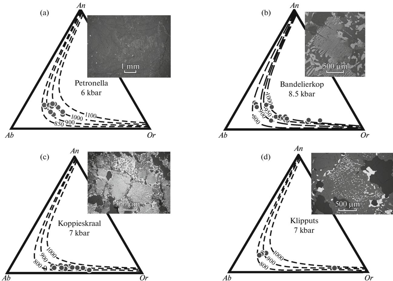
**Fig. 3.** Reintegrated compositions of feldspars from leucocratic granitoids in (a) Petronella, (b) Bandelierkop, (c) Koppieskraal, and (d) Klipputs. Isotherms are calculated based on the ternary feldspar solid solution model (Elkins and Grove, 1990). BSE images in the insets show the types of exsolution textures in feldspars of the granitoids.
