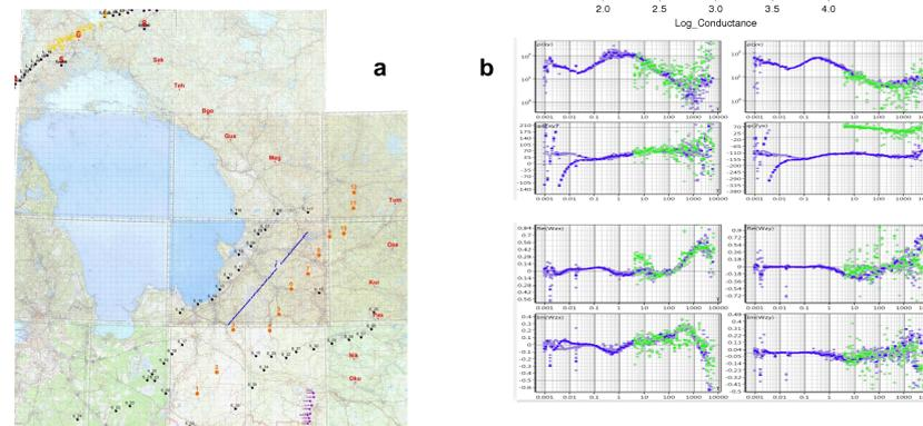
**Figure 7.** Working chart of 2018 August MT/MV campaign in ES Lake Ladoga region. 12 combined broad-band-LMT 5 component 2-days sounding have been carried out by field crew of LADOGA WG with LEMI and MERI-Pro stations (red circles 1-12 in the map of figure 7a). b - combined plot of preliminary in-field estimates of main impedances and tippers on the observations of MERI-Pro (blue dots) and LEMI (green) in site 8 (in measuring geographic axes).
