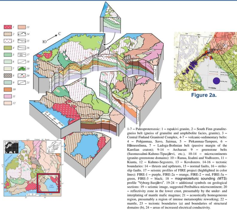
**Figure 1.** Integrated geotectonic model of SE Fennoscandian Shield, based on surface geology, reflectivity seismic data FIRE1,2,3 [Kukkonen, Lahtinen (eds.), 2006], and 4 geoelectrical profiles: SVEKA [Korja et al., 2002]; FIRE1,2 [Vaittinen et al., 2013]; LLA (Vyborg-Suojarvi profile) [Sokolova et al., 2016, 2017].
