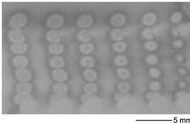
Fig. 11. Nickel substrate after depositions with total Ar flow of 500 ml/min and total  $\text{CH}_4$  flows (from left-hand side) of 0.8, 1.1, 1.5, 1.9, 2.2 and 3.0 ml/min.
