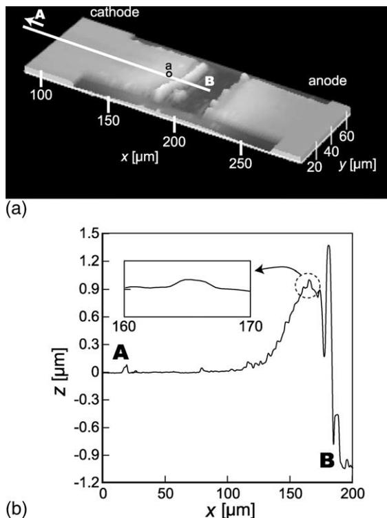
Fig. 4. Results of surface tracer measurement:  $x$ , distance;  $z$ , height. (a) Surface morphology near the gap. (b) Cross-section of the white line in (a). Level A is the cathode surface and B is the gap. The projection near  $x = 180$  results from the damaged electrode.
