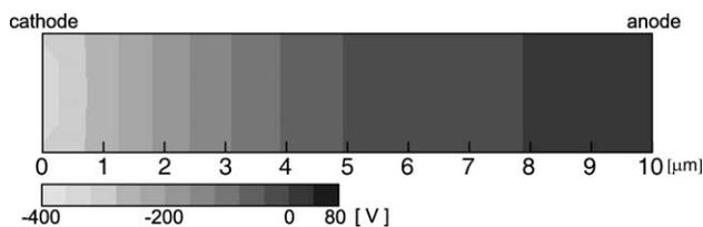
Fig. 6. Distribution of potential (10  $\mu\text{m}$  gap,  $H_2$  760 Torr, 350 V). Potentials of the cathode and anode are  $-350$  and  $0$  V, respectively.
