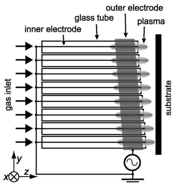
Fig. 2. Schematic diagram of multiple RF microplasma generators.
