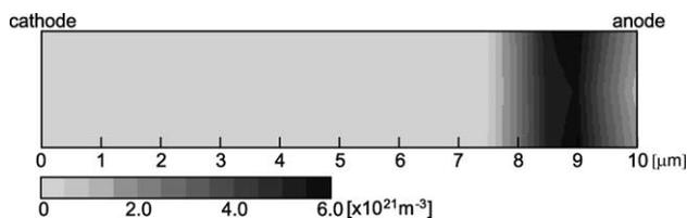
Fig. 7. Distribution of electron density (10  $\mu\text{m}$  gap,  $H_2$  760 Torr, 350 V).
