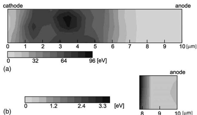
Fig. 8. Distributions of electron energy (10  $\mu\text{m}$  gap,  $\text{H}_2$  760 Torr, 350 V). (a)  $x = 0\text{--}10\ \mu\text{m}$ , (b)  $x \approx 8\text{--}10\ \mu\text{m}$ .
