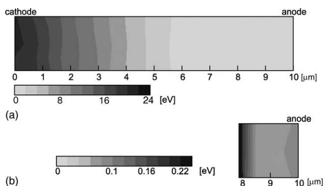
Fig. 9. Distributions of  $\text{H}_2^+$  ion energy (10  $\mu\text{m}$  gap,  $\text{H}_2$  760 Torr, 350 V). (a)  $x = 0\text{--}10\ \mu\text{m}$ , (b)  $x \approx 8\text{--}10\ \mu\text{m}$ .
