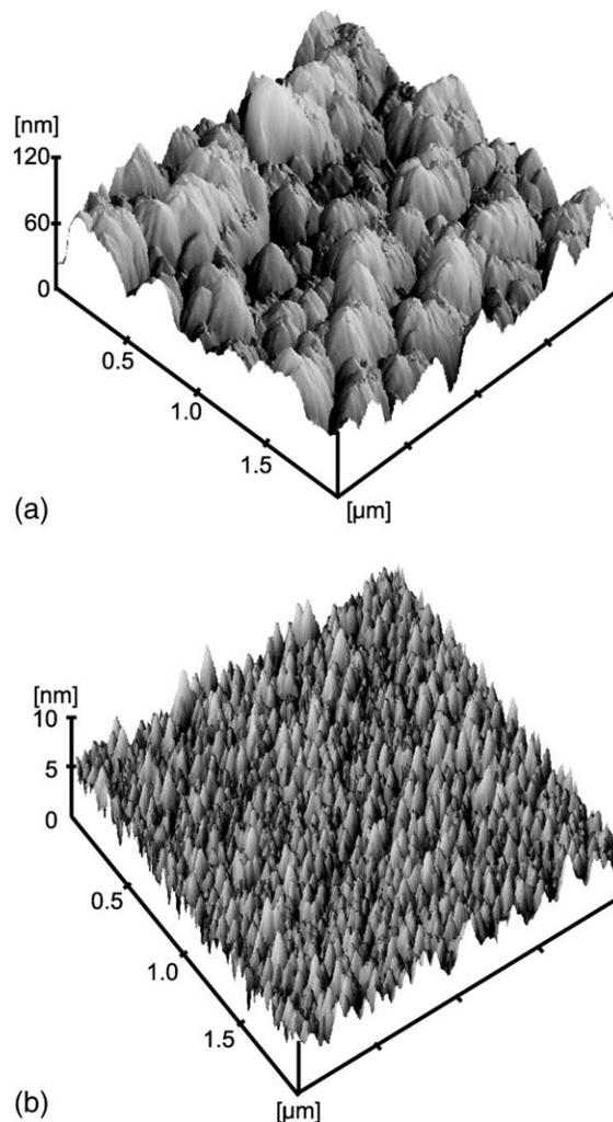
Fig. 5. (a) Surface morphology of a deposited film around the maximum film thickness region (circle a in Fig. 4(a)) measured by AFM. (b) Surface morphology of the platinum cathode that was used as the substrate.
