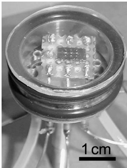
Fig. 1. Prototype plasma chip.
