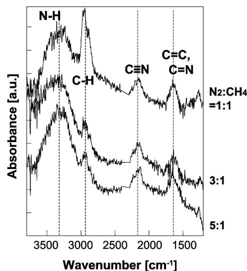
Fig. 3. Results of FT-IR measurements for the electric current of  $1.5\text{ }\mu\text{A}$ .
