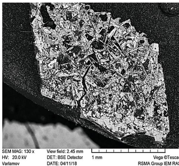
Fig. 2. Products of experiments on amphibolization of gabbro.
