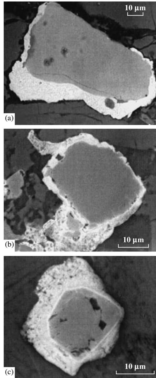
**Fig. 4.** Zonal accessory chromspinel with high-alumina core and Fe-Zn-chrommagnetite (pale) rim in lamprophyre dikes in the Chetlas Kamen Plateau, Middle Timan. Compo regime, polish section.
