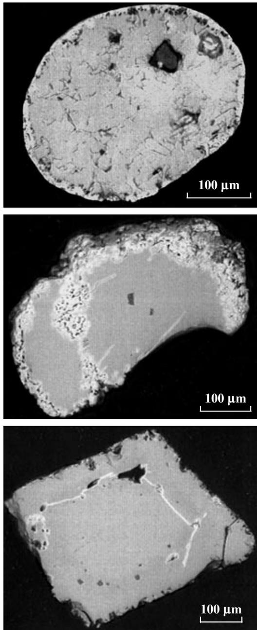
**Fig. 1.** SEM images of chromspinel from the Ichet'yu ore prospect (Vol'sk-Vymsk Range, Middle Timan). Polished sections, Compo regime. One can see partially eroded pale Zn-rich rim.
