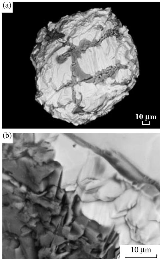
**Fig. 3.** Manganozincochromite with Cr-mica (fuchsite) inclusions. (a) Slightly polished fractured grain ( $150 \times 170 \mu\text{m}$ ); (b) closeup of (a) showing the induction surface of the joint growth of mica (dark) and manganozincochromite (pale).
