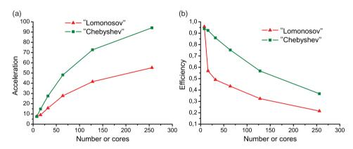
Figure 4. Acceleration (a) and efficiency (b) dependencies on number of computational cores on supercomputers 'Lomonosov' [12] and 'Chebyshev' [11].
