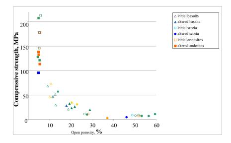
Figure 7: Dependence of uniaxial compression strength of rocks from their open porosity
