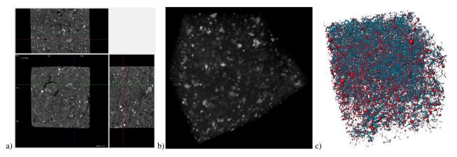
Figure 1: Images basalt samples: a) orthogonal sections (unmodified sample HK-100-1-34); b) visualization of the location of ore minerals (shown in white) in a sample of basalt HK-102-30; c) grid model pore space of basalt sample HK-102-30 (red - pores, blue - channels)
