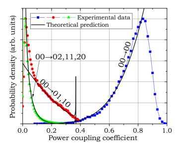
FIG. 2. Experimental results and theoretical predictions of the fundamental mode coupling into the higher-order modes.
