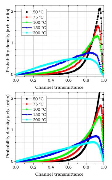
FIG. 3. Transmittance probability density for the fundamental mode: a comparison between the experimentally measured data (top) and the second-order theory predictions (bottom).
