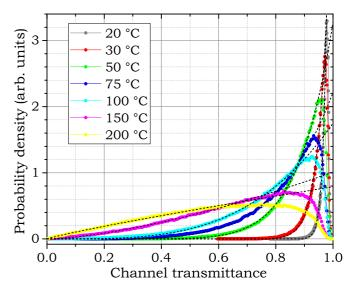
FIG. 1. Experimentally measured channel transmittance probability distribution and first-order theoretical predictions (black dashed lines). The experimental parameter governing the turbulence strength is the airflow temperature difference shown in the legend. Please note that for the better data representation probability distributions are not properly normalized.
