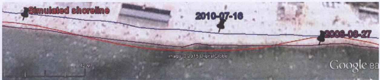
Fig. 1: A part of the simulated shoreline: red line corresponds to simulation result; blue corresponds to reference shoreline for July 16 th , 2010; magenta corresponds to initial shoreline for August 27 th , 2006.
