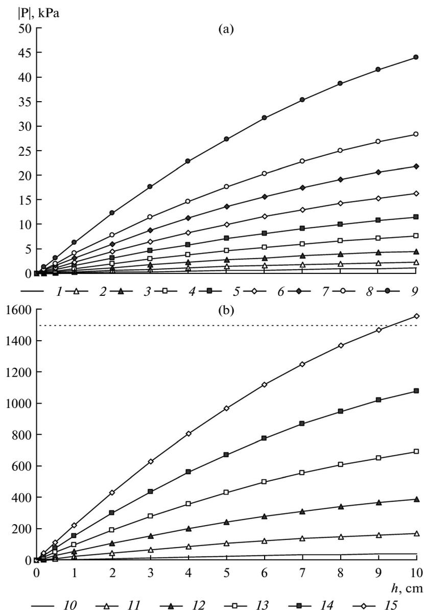
**Fig. 1.** Calculated curves of the soil water pressure as a function of the soil column height for a TsLS-3 laboratory centrifuge: (A) low centrifugation speeds (1)–(9): 100, 200, 300, 400, 500, 600, 700, 800, and 900 rpm, respectively; (B) medium and high centrifugation speeds (10)–(16): 1000, 2000, 3000, 4000, 5000, and 6000 rpm, respectively; (the dotted line) the pressure corresponding to the wilting point (1500 kPa).
