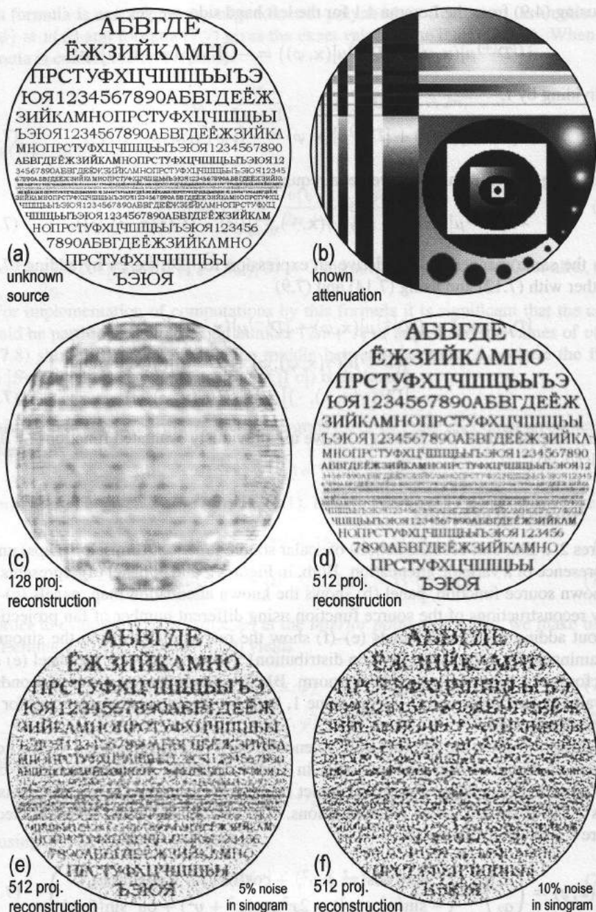
Figure 2. Reconstructions of a scalar function (a) from its attenuated Radon transform with a known attenuation map (b) without (c,d) and with (e,f) added noise
