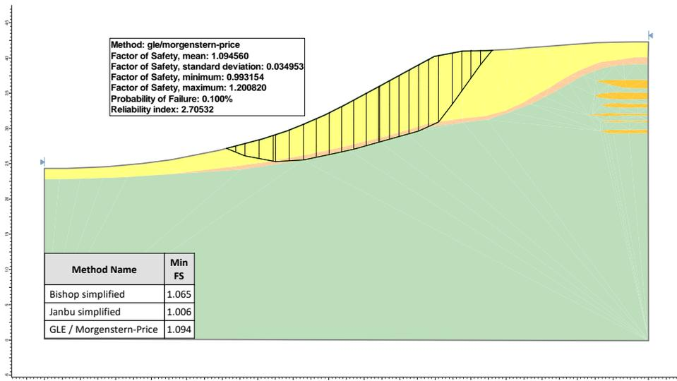
Fig. 3. Slope stability assessment with the results of probability analysis by Morgenstern-Price method (variant 2)
