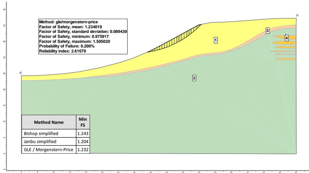
**Fig.1.** Slope stability assessment with the results of probability analysis made by Morgenstern-Price method (variant 1)
