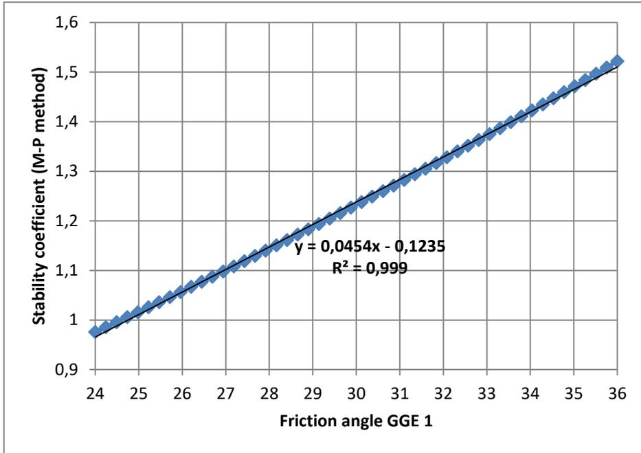
Fig. 2. The relationship between  $S_c$  and friction angle of CGE 1
