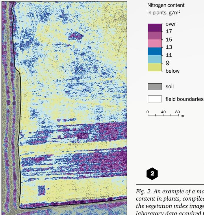
*Fig. 2. An example of a map of nitrogen content in plants, compiled on the basis of the vegetation index image calibration with laboratory data acquired from test areas*
