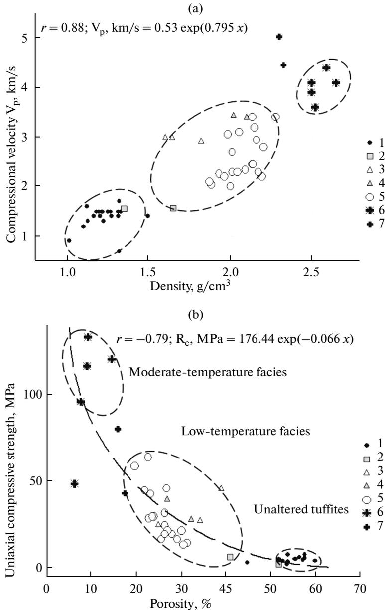
**Fig. 8.** Plots showing the compressional velocity versus density (a) and uniaxial compressive strength (b) for different rocks. (1) unaltered tuffites, (2) opal claystone, (3) mono-opalites, (4) ferrous mono-opalites, (5) low-temperature propylites, (6) moderate-temperature propylites, (7) quartz–alunite metasomatites.
