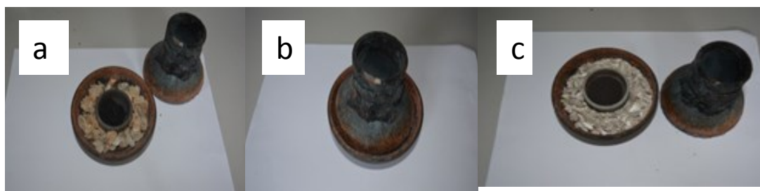
Fig.1 Before heat treatment: how the samples placed in the tool (a), closed version (b) and after heat treatment: how looked the samples (c)
