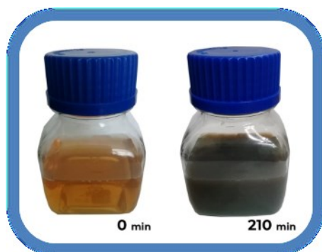
Figure 2. Color change of solution during the reaction of AgNPs synthesis.
