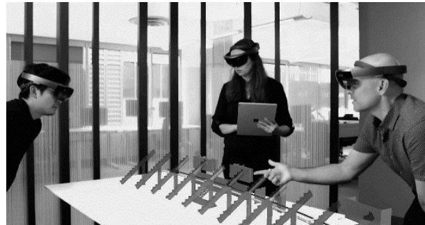
Fig. 6 Verifying the construction in AR, Bentley Synchro 4D, Image courtesy of Bentley Systems.
