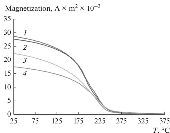
**Fig. 5.** Dependence of the magnetization of the catalysts on temperature after their activation in the synthesis gas: (1) K/Fe/C, (2) Fe/C, (3) (FeK)/C, and (4) Fe/K/C.
