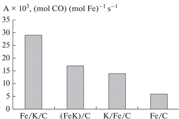
**Fig. 6.** Dependence of the specific activity on the type of catalysts.
