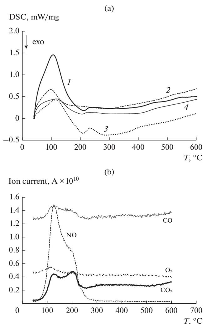
**Fig. 1.** (a) Results of the differential thermal analysis of the catalysts: (1)  $\text{Fe}(\text{NO}_3)_3 \cdot 9\text{H}_2\text{O}/\text{C}$ , (2)  $\text{KNO}_3/\text{C}$ , (3)  $(\text{Fe}(\text{NO}_3)_3 \cdot 9\text{H}_2\text{O} + \text{KNO}_3)/\text{C}$ , and (4)  $(\text{Fe}(\text{NO}_3)_3 \cdot 9\text{H}_2\text{O}/\text{K}/\text{C})$ . (b) The mass spectrum of gases released in the course of the DTA of the Fe/C catalyst.
