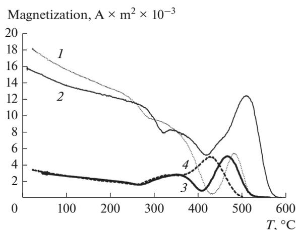
**Fig. 4.** Dependence of the magnetization on temperature in the course of catalyst activation in synthesis gas: (1) K/Fe/C, (2) Fe/C, (3) (FeK)/C, and (4) Fe/K/C.
