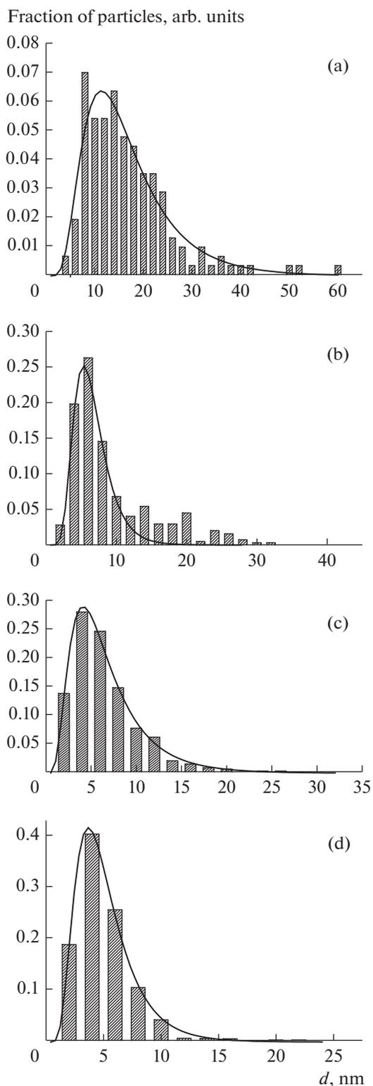
**Fig. 2.** Histograms of the particle size distributions based on the transmission electron microscopy data: (a) Fe/C, (b) K/Fe/C, (c) (FeK)/C, and (d) Fe/K/C.
