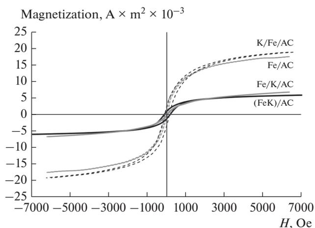
**Fig. 3.** Dependence of the magnetization on the field intensity for the initial catalysts.
