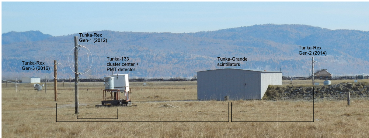
Figure 6. Photo of a single cosmic-ray cluster of the TAIGA facility. Lines mark the cable connections between Tunka-Rex antennas and the DAQ of Tunka-133 and Tunka-Grande.
