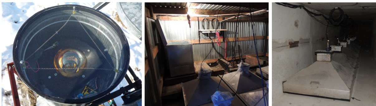
Figure 7. Photo of the interior of a Tunka-133 optical module ( left ), on-ground ( center ) and underground ( right ) Tunka-Grande scintillators.
