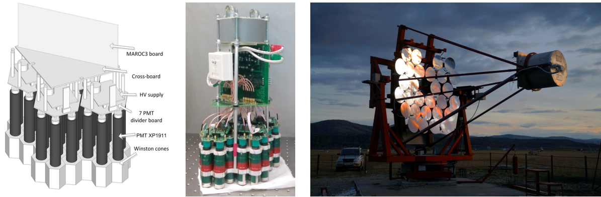
Figure 11. Left and center: Design and photo of a TAIGA-IAC T camera cluster, which contains 28 PMTs and an independent board generating the trigger. Right: Photo of the first TAIGA-IAC T telescope with 29 mirror segments installed.
