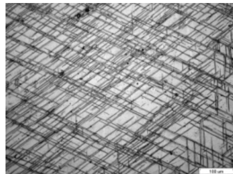
Figure 2. Microstructure of Mg single crystal samples of c -orientation recovered after shock loading.
