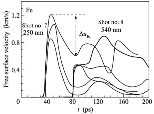
**Fig. 6.** Evolution of the compression wave in iron in the range from 250 to 540 nm at the energy density varying from 2.5 J/cm<sup>2</sup> in the center to 0.8 J/cm<sup>2</sup> in the peripheral part of the focal spot.
