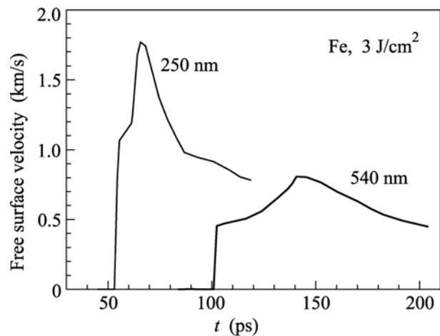
**Fig. 4.** Evolution of the compression pulses propagating in iron.
