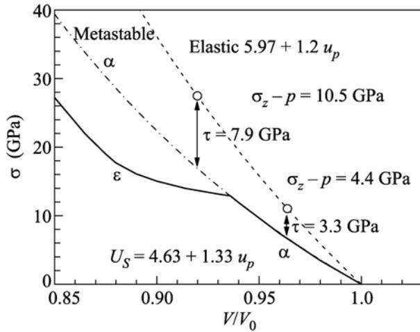
**Fig. 5.** Parameters of the state of iron behind the shock precursor front at distances of 250 and 540 nm.
