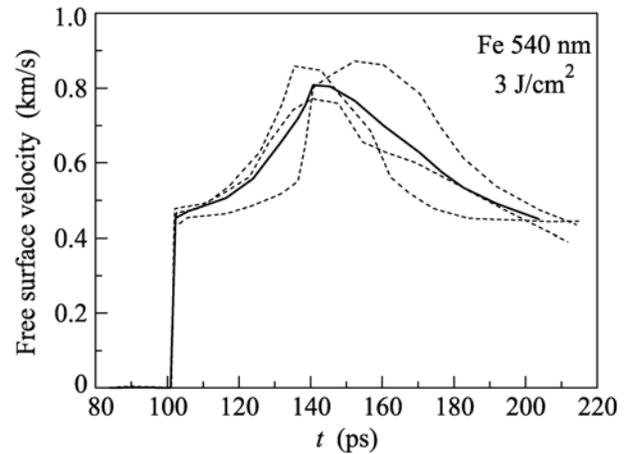
**Fig. 3.** (Dashed lines) Velocity profiles of the free surface of the 540-nm-thick film sample at an energy density of  $3 \text{ J/cm}^2$ . The wave fronts are shifted from the average motion beginning time by no more than 1 ps. The solid line is the averaged profile  $u_{fs}(t)$ .
