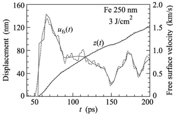
**Fig. 2.** Example of the processing of one of the displacement profiles  $z(t)$  shown in Fig. 1 for the 250-nm-thick sample. The dashed lines are the measured displacement profile and the velocity profile of the free surface obtained by the differentiation of the smoothed profile  $z(t)$ . The solid lines are obtained by iterative processing.
