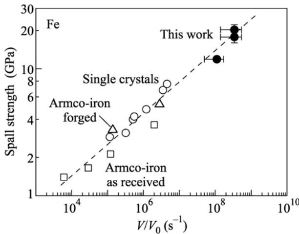
Fig. 7. Spall strength of iron measured for picosecond loads in comparison with the data obtained in the experiments with colliding plates [24].
