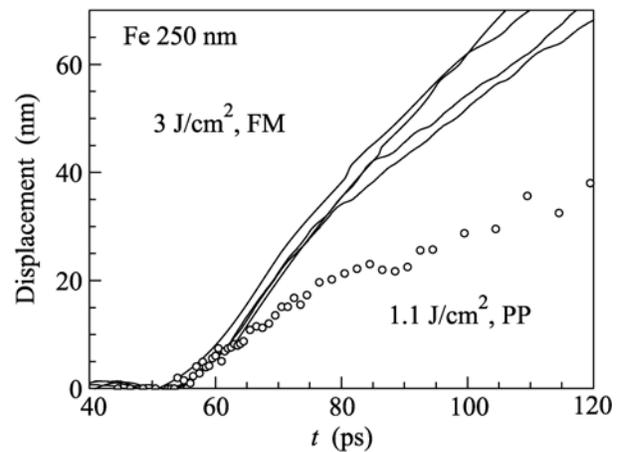
**Fig. 1.** Displacement histories of the free rear surface of the iron film sample as measured with the use of the (lines, FM) frequency-modulated pulse and (points, PP) pump–probe method at the energy densities of 3 and  $1.1\ \text{J}/\text{cm}^2$ , respectively, in the center of the focal spot. Here and below, zero time is chosen arbitrarily.
