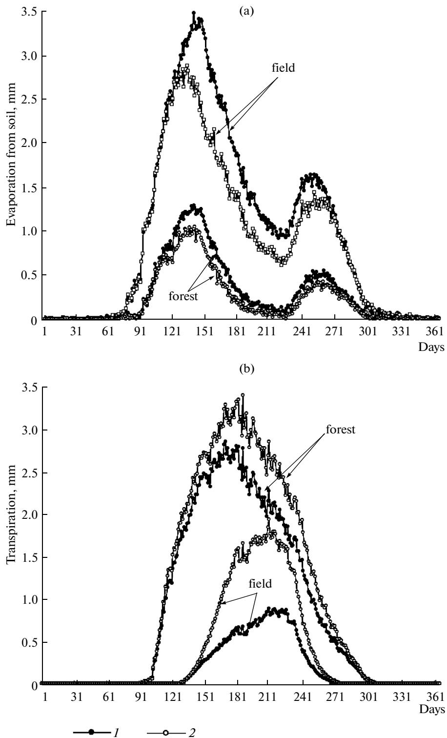
**Fig. 3.** Annual dynamics of daily (a) evaporation from soil and (b) transpiration for different landscape and geological-pedological conditions at deep GWT (here and in Fig. 4, (I) loams, (2) sands).
