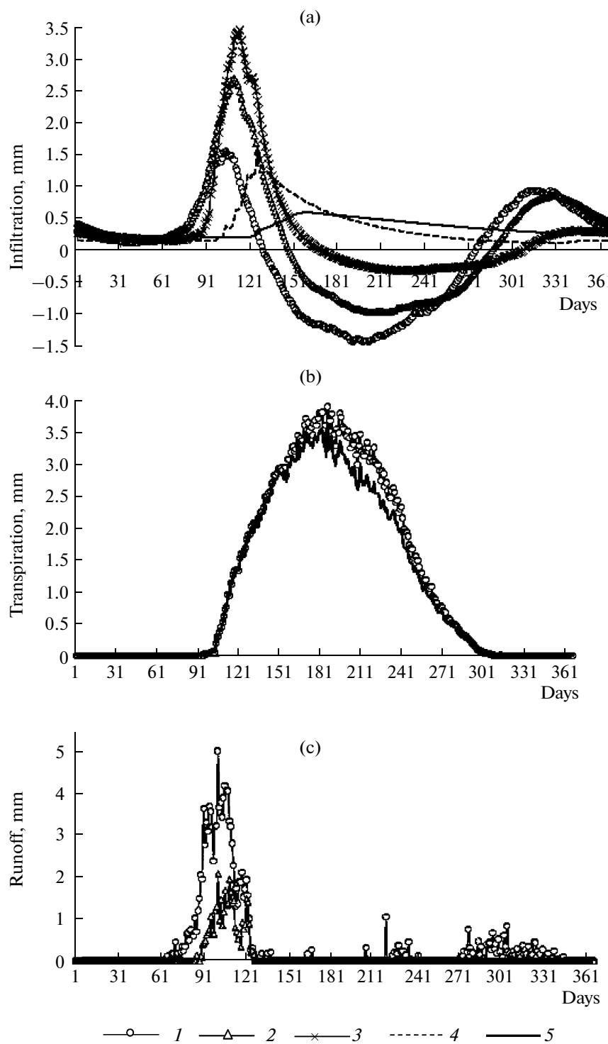
**Fig. 6.** Annual dynamics of water balance components for vadose zone: (a) infiltration, (b) transpiration, (c) surface runoff at different depth to GWT for forest sandy loam-loamy soil. Depth to GWT: (1) 0.5 m, (2) 1, (3) 2, (4) 4, (5) 6 m.
