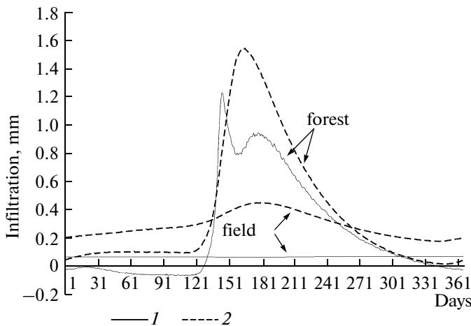
**Fig. 4.** Within-year dynamics of daily infiltration rates for different landscape and geological-pedological conditions at deep GWT.
