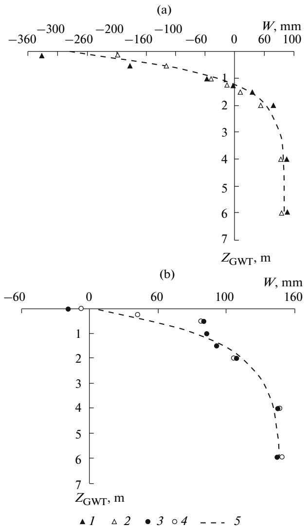
**Fig. 5.** Typical calculated dependence of infiltration  $W$  on the depth to GWT  $Z_{\text{GWT}}$  for (a) loam sand and (b) sand bed for the case of a forest landscape. (1) Loamy sand, (2) loamy sand overlying clay, (3) sand, (4) sand on sandy loams, (5) approximating curve.
