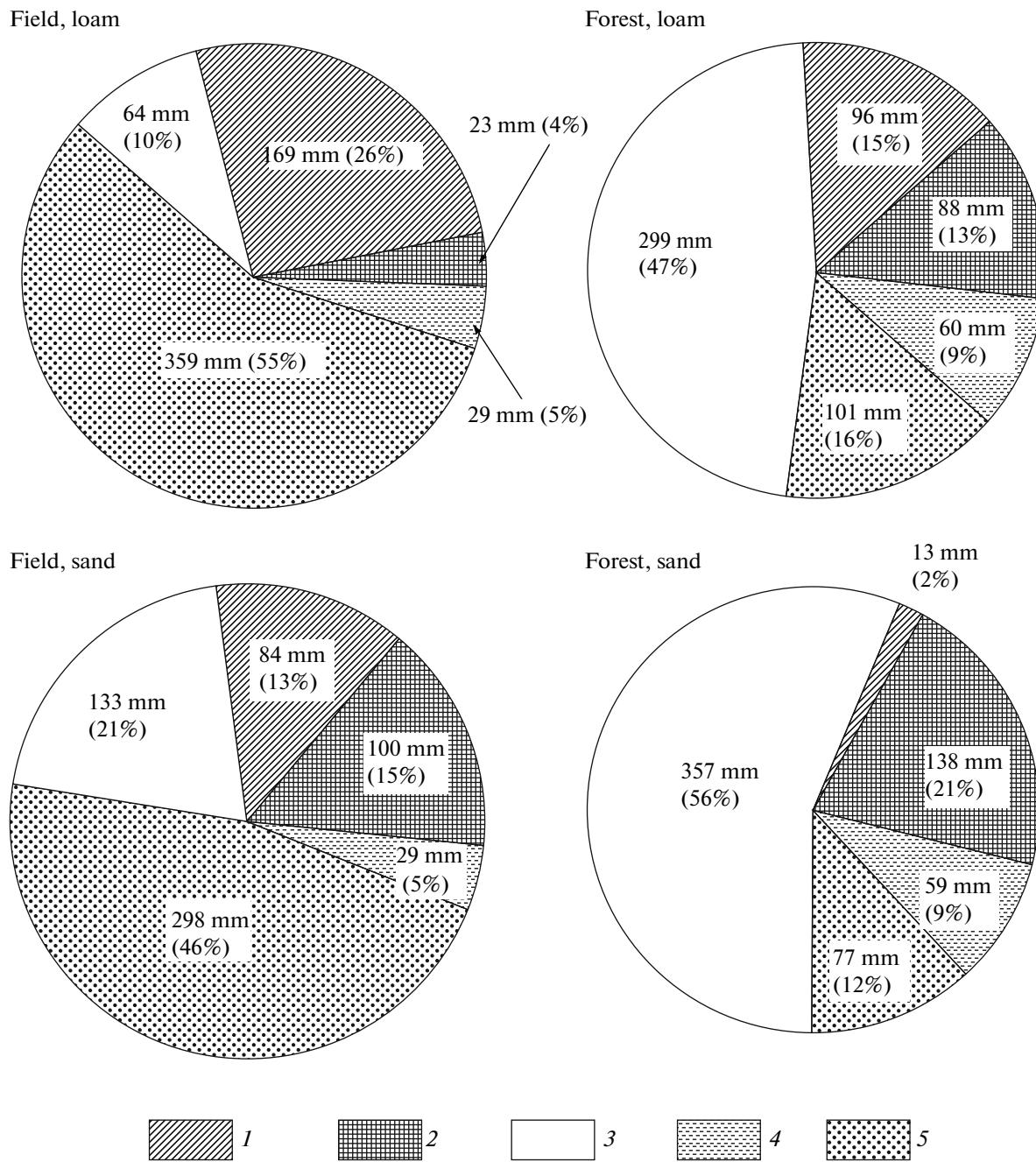
**Fig. 7.** Comparison of calculated characteristics of annual water balance, mm of depth and % of precipitation, for different landscape and geological-pedological conditions at deep GWT. (1) surface runoff, (2) infiltration, (3) transpiration, (4) surface evaporation, (5) evaporation from soil.
