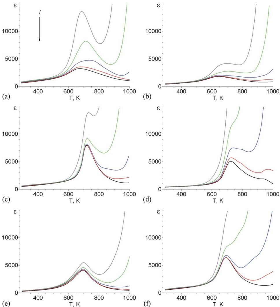
**Figure 3.** Dielectric permittivity versus temperature curves (cooling) of modified BSPT ceramics: (a) II (10 w.% BTO); (b) IV (10 w.% BSO) prepared at  $T_1 = 973$  K (7 h),  $T_2 = 1323$  K (1 h),  $T_3 = 1473$  K (1 h),  $T_4 = 1073$  K (1 h); (c) I (5 w.% BTO) + 1 w.% LiF; (d) II (5 w.% BSO) + 1 w.% LiF; (e) II (10 w.% BTO) + 1 w.% LiF; (f) IV (10 w.% BSO) + 1 w.% LiF prepared at  $T_1 = 973$  K (7 h),  $T_2 = 1473$  K (1 h). Measuring frequencies: 100 Hz, 1 kHz, 10 kHz, 100 kHz, 1 MHz.
