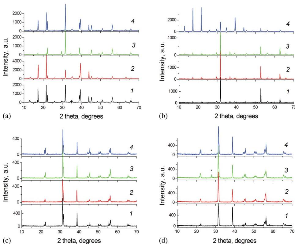
**Figure 1.** X-ray diffraction patterns of ceramic samples I–IV prepared at: (a)  $T_1 = 973$  K;  $T_2 = 1223$  K (1 h),  $T_3 = 1423$  K (1 h); (b)  $T_1 = 973$  K;  $T_2 = 1223$  K (1 h),  $T_3 = 1473$  K (1 h); compositions I–IV with 1 w.% LiF additive prepared at: (c)  $T_1 = 973$  K;  $T_2 = 1223$  K (1 h); (d)  $T_1 = 973$  K;  $T_2 = 1473$  K (1 h) (Figure available in color online).
