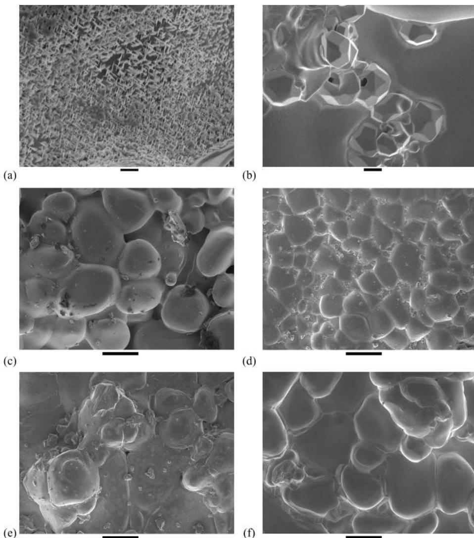
**Figure 2.** SEM images of surfaces of modified BSPT ceramics: (a) II (10 w.% BTO) prepared at  $T_1 = 973$  K (7 h),  $T_2 = 1323$  K (1 h),  $T_3 = 1473$  K (1 h),  $T_4 = 1073$  K (1 h); (b) IV (10 w.% BSO) + 1 w.% LiF; (c) I (5 w.% BTO) + 1 w.% LiF; (d) II (10 w.% BTO) + 1 w.% LiF; (e) III (5 w.% BSO) + 1 w.% LiF; (f) IV (10 w.% BSO) + 1 w.% LiF prepared at  $T_1 = 973$  K (7 h),  $T_2 = 1473$  K (1 h). Black bars denote  $1 \mu\text{m}$  (a, b) and  $10 \mu\text{m}$  (c-f).
