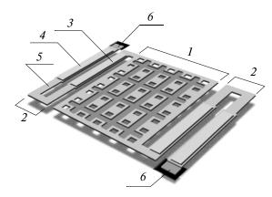
Fig. 1. Design of the sensitive element of the uncooled MOMS IR matrix: (1) receiving membrane; (2) microconsoles; (3, 4) main and compensating bimaterial segments of the microconsole, respectively; (5) thermal insulation segment; and (6) places of microconsole fastening to the substrate (anchor). Sizes of the sensitive element are  $50 \times 50 \ \mu m$ .
