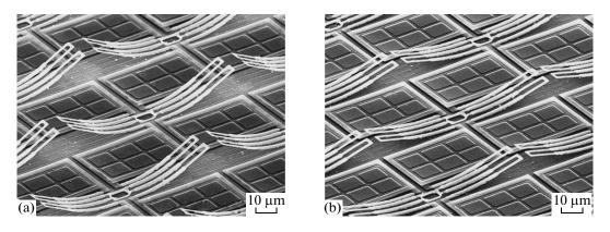
**Fig. 4.** SEM image of the bimaterial MOMS IR detector with the thermal compensation at the substrate temperature of (a)  $-24^{\circ}$ C and (b)  $+150^{\circ}$ C.
