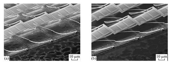
Fig. 3. SEM image of the bimaterial MOMS IR detector with elongated microconsoles at the substrate temperature of (a)  $-24^{\circ}$ C and (b)  $+150^{\circ}$ C.
