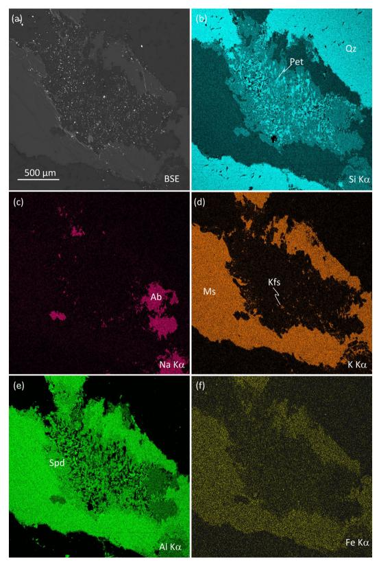
**Fig. 13**. EDS elemental mapping of a representative rock domain involving spodumene, quartz, petalite, albite, muscovite and K-feldspar. (**a**) BSE image, (**b**) Si Kα, (**c**) Na Kα, (**d**) K Kα, (**e**) Al Kα, (**f**) Fe Kα. Petalite is restricted to spodumene and quartz and does not occur along the interface of muscovite or albite.
