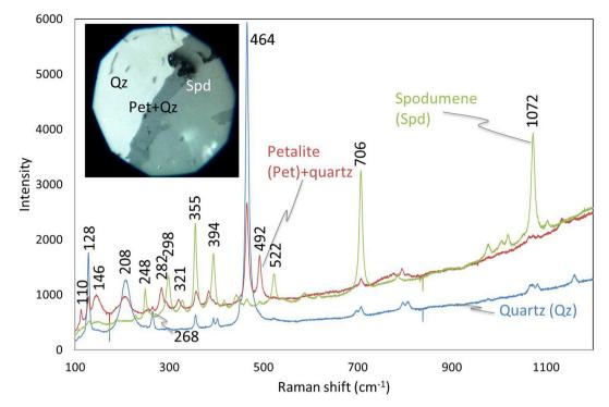
Fig. 9. Raman spectra of quartz (Qz), spodumene (Spd) and petalite + quartz (Pet+Qz) obtained across the reaction zone shown in the reflected light image in the inset (quartz – bright, petalite + quartz – dark grey, spodumene – medium grey).
