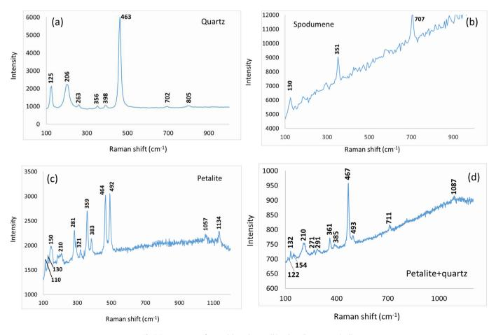
Fig. 8. Raman spectra of quartz (a), spodumene (b) and petalite + quartz (c, d).
