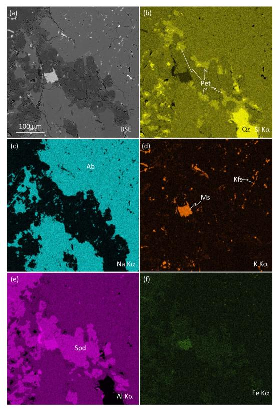
**Fig. 11**. EDS elemental mapping of a representative rock domain involving spodumene, quartz, petalite, albite, muscovite and K-feldspar. (a) BSE image, (b) Si Kα, (c) Na Kα, (d) K Kα, (e) Al Kα, (f) Fe Kα. The petalite rims conspicuously follow the margin of spodumene. Note that the muscovite is separated from petalite by spodumene [better seen in (b)].
