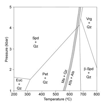
**Fig. 1.** Pressure-temperature diagram showing phase boundaries of the system LiAlSiO<sub>4</sub>-SiO<sub>2</sub>-H<sub>2</sub>O [from London, 1984]. Equilibria curves showing the break-down of muscovite + quartz (muscovite + quartz = K-feldspar + Al<sub>2</sub>SiO<sub>5</sub> + H<sub>2</sub>O) from Kerrick (1972) is also shown. Spd – spodumene; Vrg – virgilite; Euc – eucryptite; Pet – petalite; Qz – quartz; Ms – muscovite; Als – aluminosilicate.
