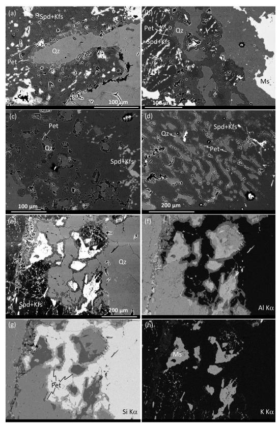
**Fig. 7.** BSE images (**a to e**) illustrating the textural relation between spodumene, quartz (Qz) and petalite (Pet) from the spodumene pegmatites. (**f to h**) EDS elemental mapping of a representative textural domain (e) is shown, with elements Al Kα (f), Si Kα (g) and K Kα (h) shown.
