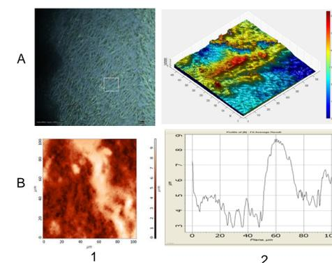
Figure 4. Investigation of the morphology of chitosan thin films containing fibroin. A – Modulation interference microscopy: optical (1) and 3D-phase (2) images of the surface. B - Atomic Force Microscopy: image (1) and surface micro-profile (2).
