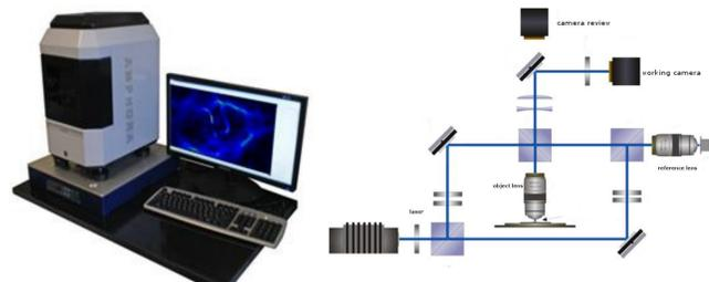
Figure 1. Computer Phase-Interference Microscope
