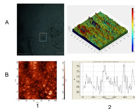
Figure 5. Investigation of the surface morphology of chitosan thin films cross-linked with jenipine and containing fibroin (1:1). A – Modulation interference microscopy: optical (1) and 3D-phase (2) images of the surface. B - Atomic Force Microscopy: image (1) and surface micro-profile (2).
