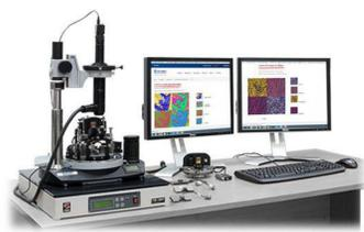
Figure 2. Atomic force Microscopy based on the NtegraPrima
