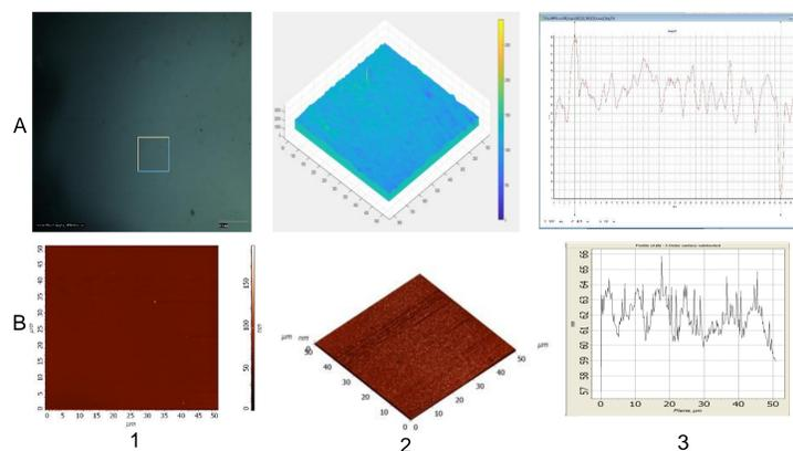
Figure 3. A – Modulation interference microscopy; B - Atomic Force Microscopy. 1 - visualizing the surface; 2 - evaluation of surface geometric parameters; 3 - averaged surface roughness index.
