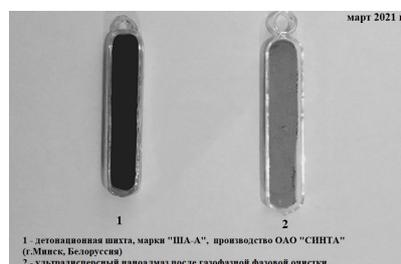
Fig.1 Sample of detonation nanodiamond grade "SHA-A": 1 - before processing; 2 - DNA obtained after gas-phase phase cleaning, used in de-icer
