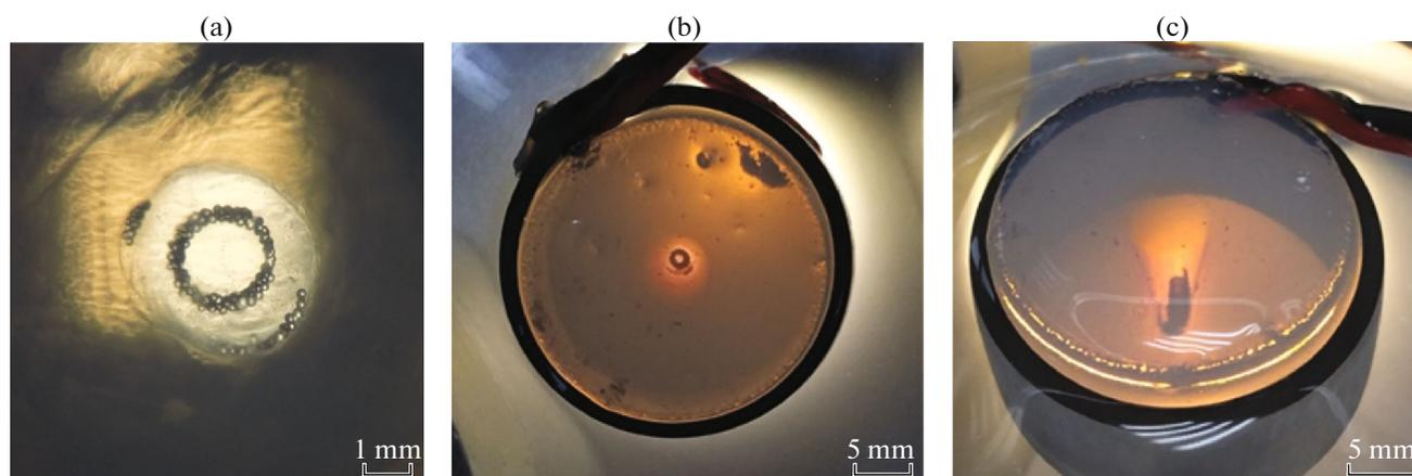
**Fig. 2.** Photographs of the experiment. (a) Top view: tube of polystyrene balls mimicking tissue spheroids; (b) top and (c) angle views of a tube made from chondrospheres in an agarose container inside a piezocylinder. The unit was immersed in a nutrient solution.
