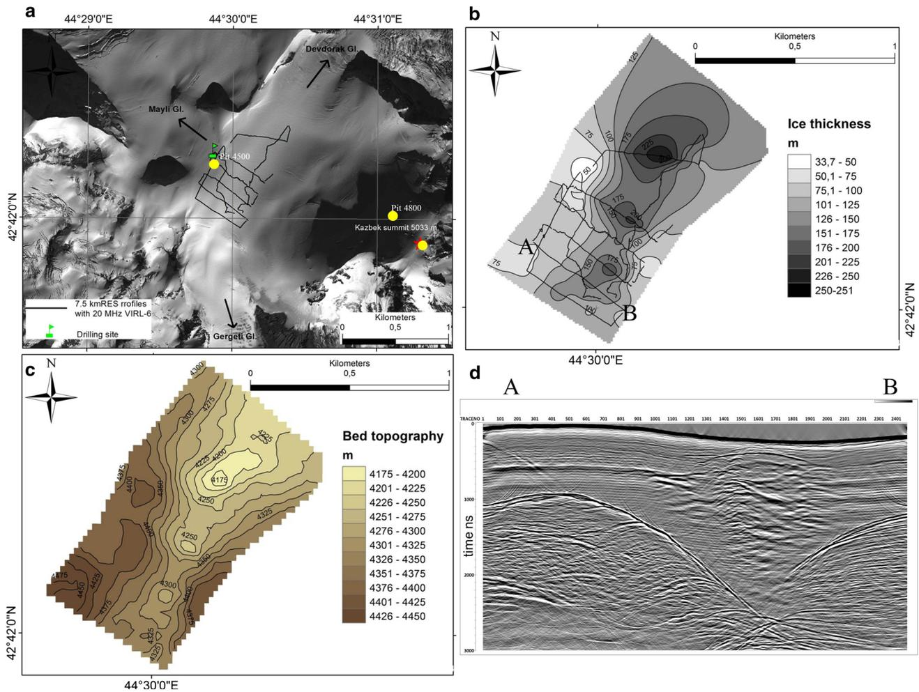
**Fig. 3** Location of the shallow drilling site on the Kazbek plateau (4500 m) and GPR survey profiles obtained during the 2014 field season are shown (a). Glacier thickness and the relief of the basement
