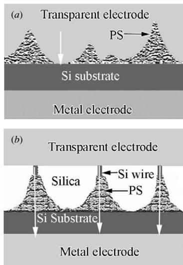
**Figure 4.** Schematic drawing of electric contacts in devices fabricated on top of (a) normal PS and (b) PS connected with silicon wires.
