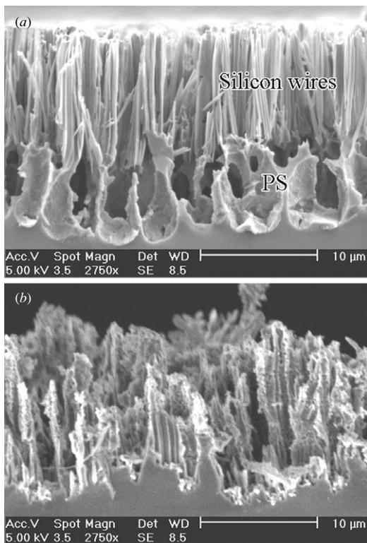
**Figure 2.** Different structures after electrochemical anodization (a) porous silicon covered with silicon wires by using thinner silicon wires; (b) PS-covered wires by using thicker (over 1  $\mu\text{m}$  in diameter) Si wires.
