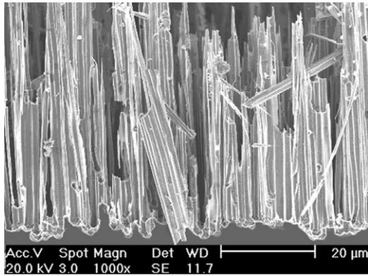
**Figure 1.** Silicon wires obtained by one-step chemical etching.
