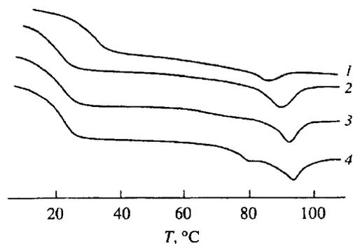
**Figure 2.** DSC curves for the copolymers  $C_1$  (1),  $C_3$  (2), and for chiral mixtures  $C_2\text{-Mt-}5.6$  (3),  $C_3\text{-Mt-}11$  (4).
