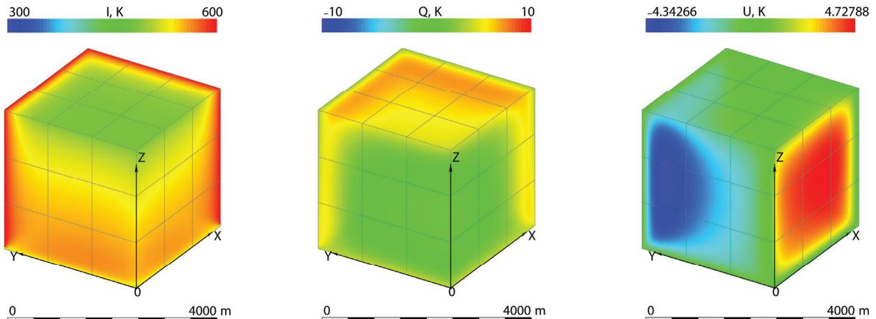
FIGURE 2. 3D rain cell view projection. Wave length  $\lambda = 3$  mm, rain intensity 20 mm/h, lambertian reflectance  $R = 0.25$
