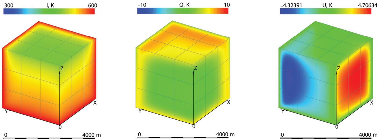
FIGURE 1. 3D rain cell view projection. Wave length  $\lambda = 3$  mm, rain intensity 20 mm/h, lambertian reflectance  $R = 0$ .
