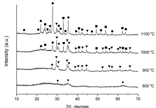
**Fig. 1.** XRD patterns of Zr0 fiber annealed at 800, 900, 1000 and 1100 °C for 24 h in air (◆ – magnesioferrite, ▼ – pyroxene, ● – plagioclase, ■ – hematite).
