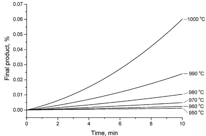
**Fig. 7.** Isotherms of plagioclase crystallization versus time for Zr0 fiber in air.
