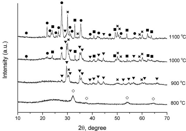
**Fig. 2.** XRD patterns of Zr5 fiber annealed at 800, 900, 1000 and 1100 °C for 24 h in air ( $\diamond$  – cubic complex oxide  $MO_x$ , where  $M = Mg, Zr, Ti$ ,  $\times$  – tetragonal  $ZrO_2$ ,  $\blacktriangledown$  – pyroxene,  $\bullet$  – plagioclase,  $\blacksquare$  – hematite).
