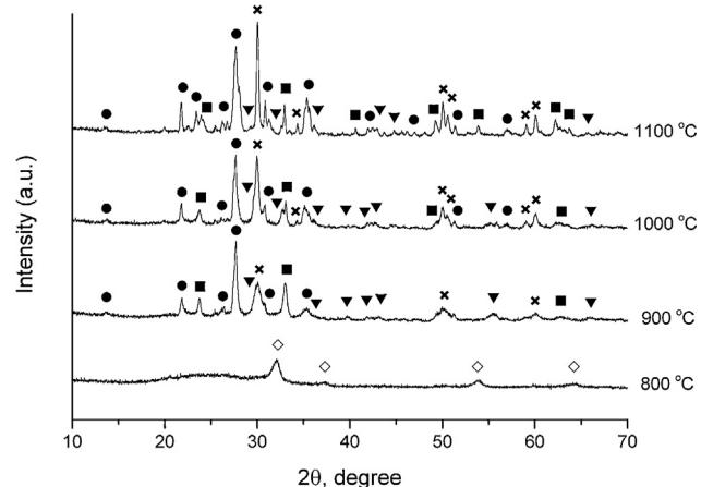
**Fig. 3.** XRD patterns of Zr7 fiber annealed at 800, 900, 1000 and 1100 °C for 24 h in air ( $\diamond$  – cubic complex oxide  $MO_x$ , where  $M = Mg, Zr, Ti$ ,  $\times$  – tetragonal  $ZrO_2$ ,  $\blacktriangledown$  – pyroxene,  $\bullet$  – plagioclase,  $\blacksquare$  – hematite).
