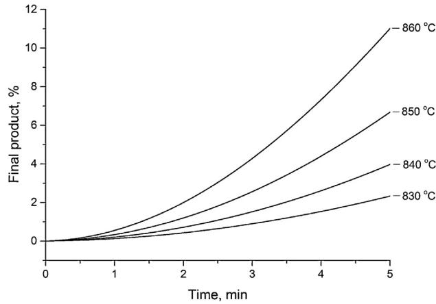
**Fig. 6.** Isotherms of pyroxene crystallization versus time for Zr0 fiber in air.
