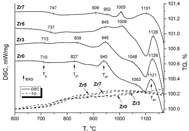
**Fig. 4.** DSC (solid line) and TG (dash line) curves of fibers with different zirconia contents in air at heating rate of 20 K/min ( $T_g$  – glass transition temperature;  $T_{p1}$ ,  $T_{p2}$ ,  $T_{p3}$  – exothermal peak temperatures).
