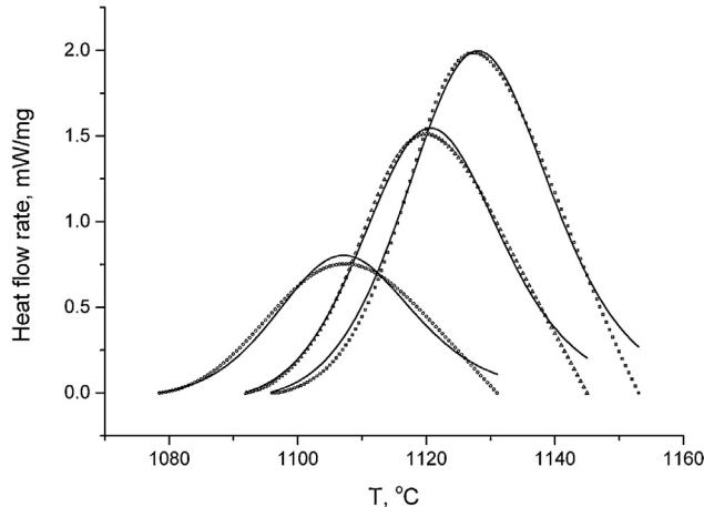
**Fig. 5.** Graphical comparison of the computation results (solid line) and experimental data (symbols) for DSC curves of plagioclase crystallization in Zr0 basalt fibers. Three heating rates (10, 20, 30 K/min); one-step reaction; the Prout–Tompkins equation.
