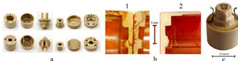
Figure 1. a – The appearance of small-sized parts; b – comparison of imperfection degree of the part made of pressing moulding material AG-4V (1) and injection moulding material TERMORAN PPS GF-40 (2) using the color capillary defectoscopy method; c – the appearance of the power source for electronic-mechanical devices.
