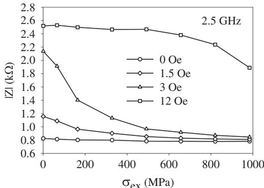
**Fig. 2.** Experimental spectra of the impedance magnitude vs. external tensile stress in  $\text{Co}_{68.5}\text{Mn}_{6.5}\text{Si}_{10}\text{B}_{15}$  amorphous glass-coated wires having the total diameter of 14.5  $\mu\text{m}$  and the metallic core diameter of 10.2  $\mu\text{m}$ . The frequency is 2.5 GHz [7].
