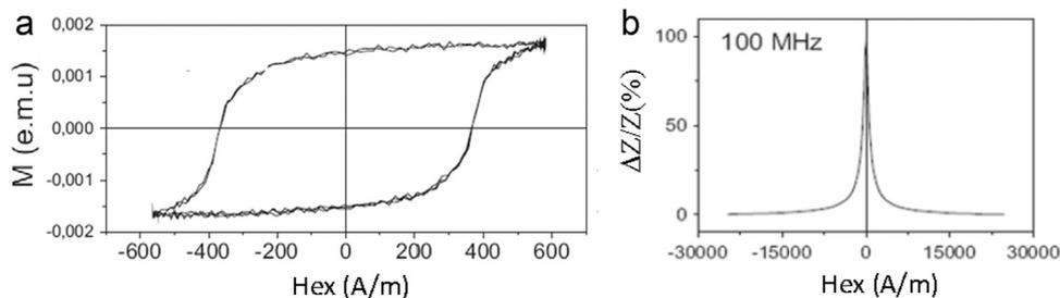
**Fig. 5.** Hysteresis loops (a) and the impedance vs.  $H_{ex}$  at 100 MHz (b) for a microwire of the composition  $\text{Co}_{57.33}\text{Fe}_{4.7}\text{Cr}_{13.4}\text{B}_{13.02}\text{Si}_{11.09}\text{Mo}_{0.62}$  with  $T_c \approx 100^\circ\text{C}$ . The total diameter is  $34.2 \mu\text{m}$  and the metal core diameter is  $30 \mu\text{m}$ .
