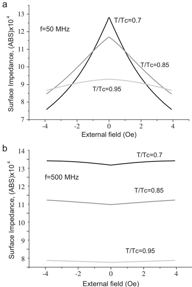
**Fig. 7.** Absolute value of the axial component of the surface impedance vs.  $H_{ex}$  for frequencies of 50 MHz (a) and 0.5 GHz (b) with a temperature as a parameter. The magnetic parameters of calculation are the same as for Fig. 6.  $a = 10$   $\mu\text{m}$ .
