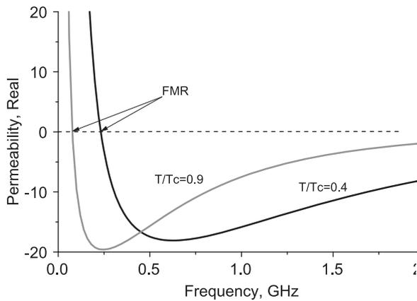
**Fig. 6.** Modelled permeability spectra (real part) for different temperatures in wires with axial anisotropy. the parameters for calculation:  $M_s = 435$  G, the anisotropy field at zero temperature  $H_K(T = 0) = 5$  Oe.
