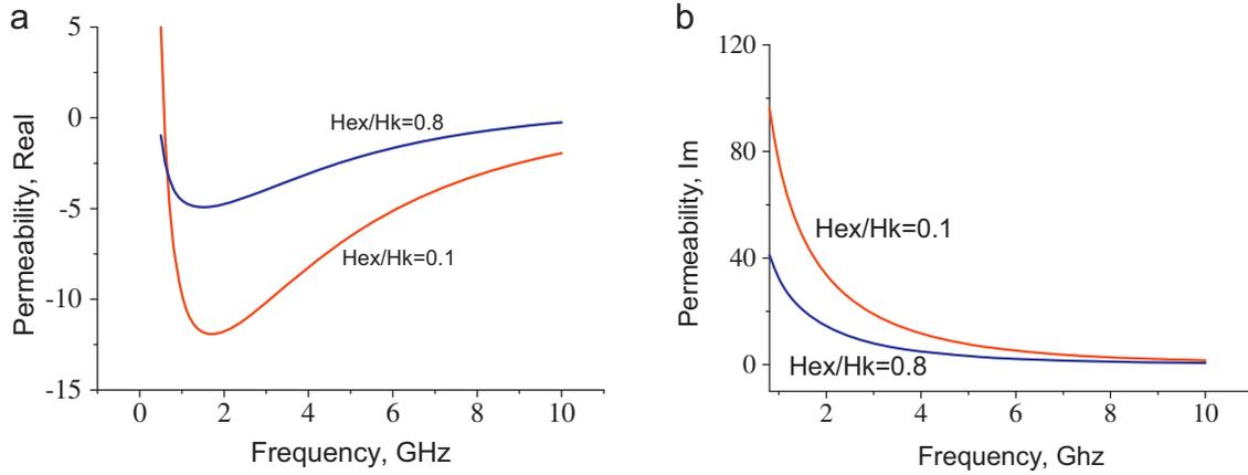
**Fig. 3.** Modelled permeability spectra of a wire with a circumferential anisotropy: (a) real part, and (b) imaginary part. The effect of a dc magnetic field  $H_{ex}$  is demonstrated. The magnetic parameters for calculation are the same as for Fig. 1. The wire resistivity is  $130 \mu\Omega \text{ cm}$ , the wire radius  $a = 5 \mu\text{m}$ .
