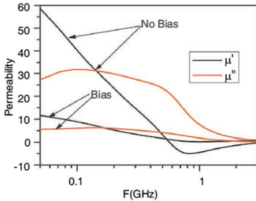
**Fig. 4.** Experimental spectra of the effective permeability of composites with 8% concentration of CoFeNiSiB amorphous wires having a diameter of  $5 \mu\text{m}$  [41]. The measurements were done with co-axial transmission line method. The effect of a bias dc magnetic field of about 200 G applied along the wires is shown. Measurements are performed in a co-axial waveguide (reproduced courtesy of The Electromagnetics Academy).
