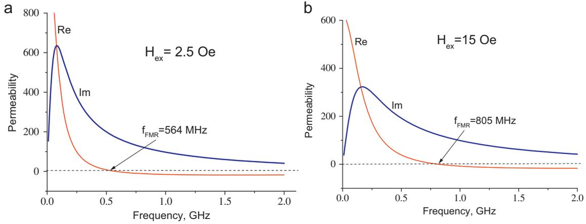
**Fig. 1.** Spectra of the permeability parameter  $\bar{\mu}$  defined by Eq. (10) in wires with a circumferential anisotropy. Parameters used for calculations: anisotropy field  $H_k = 5$  Oe,  $M_0 = 500$  G, spin relaxation parameter is 0.2. Small deviations of the anisotropy angle  $\alpha$  are used to avoid permeability divergence near a critical field of the rotational magnetisation flip.
