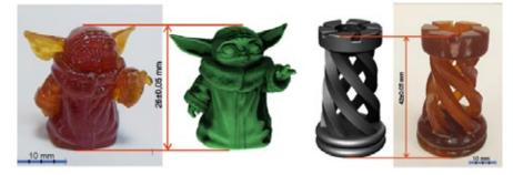
Figure 1. Digital models and 3D-objects fabricated from developed UV-curable resins.
