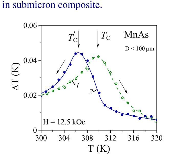
• It is established that the optimum properties, such as giant MCE and low temperature hysteresis, are found in composite with  $1\mu m$  particles and polyvinyl acetate matrix hardened at pressure of 10kBar. The maximum of MCE in this composite is  $\Delta T \sim$ 1.3 K (at 309 K) in 12.5 kOe. At the same time the temperature hysteresis of MCE is depressed. These properties are caused by the residual pressure of polymer mould on grains.
