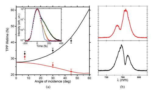
Fig. 1. a) Measured (dots) and calculated (solid curves) dependence of TPP lifetime on angle of incidence for s- (black) and p- (red) polarized light. Inset: measured cross-correlation functions of laser pulses reflected from the sample at 45° for s- (black dots) and p- (red dots) polarization of incident radiation. Blue solid curve corresponds to the auto-correlation function of the incident pulse. b) Spectra of s- (black) and p- (red) polarized laser pulses reflected from the sample.
