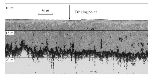
Fig. 3. A record by the high-resolution seismic profilograph obtained in the shallow part of the East Arctic sea shelf.
