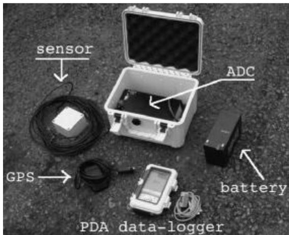
Figure 3. Portable seismic station Cossack Ranger.
