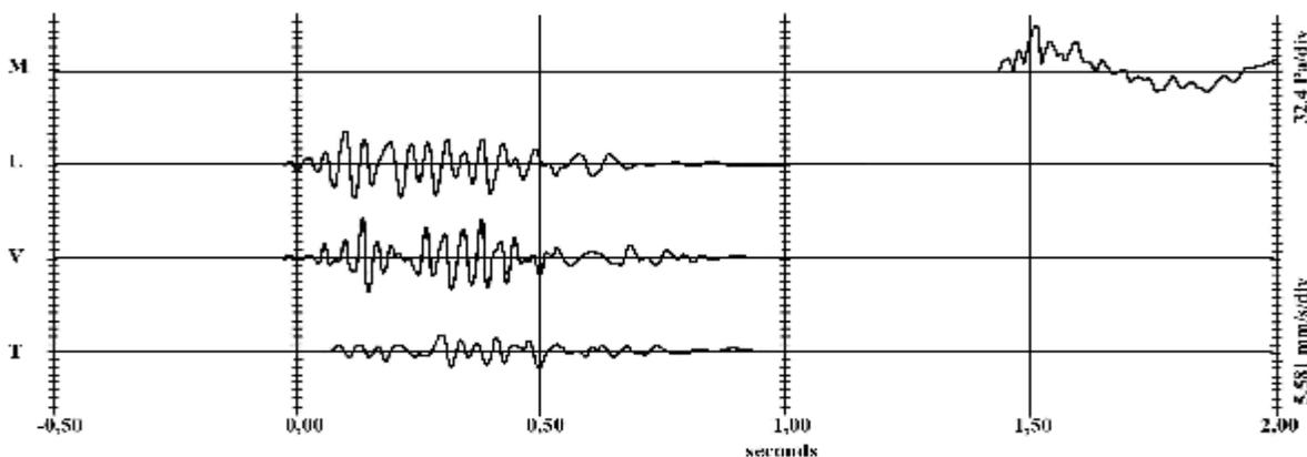
Figure 8. Record of explosion in the open pit: M - acoustic component (extra pressure); L, V and T – seismic components (velocity).
