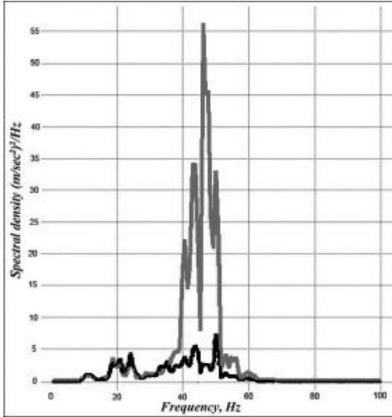
Figure 6. Spectrum of the radial component of acceleration for the seismic event on 24.10.03. Grey line – rock, black line – snow.
