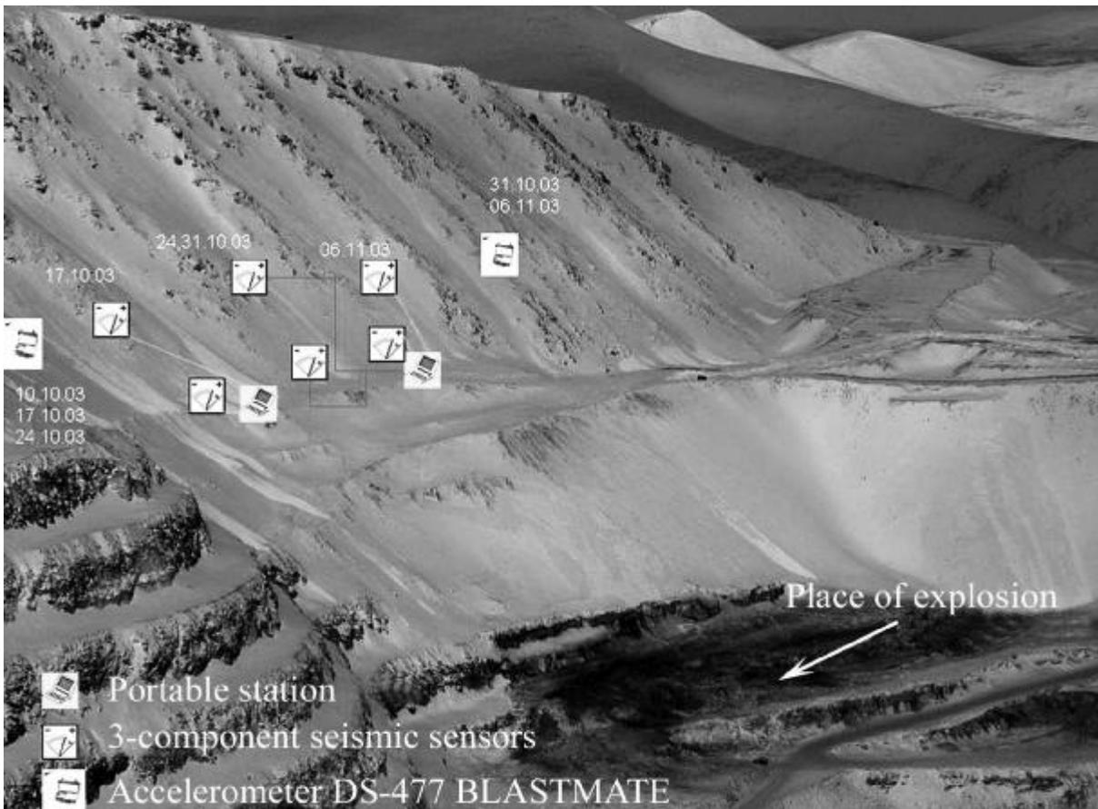
Figure 2. Picture of the avalanche sites with places of measurement sites and a part of the Central open pit mine with places of explosions.
