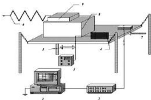
Figure 10. A sketch of the installation for simulation of seismic vibration and its influence on snow shear strength. 1. Computer; 2. ADC; 3. Frequency regulator; 4. Vibrator; 5. Periodic oscillations; 6. Constant shear load; 7. Short impulse shock load; 8. Snow block; 9. Shear frame; 10. Seismic sensor (accelerometer). It is also possible to simulate static and dynamic normal loading.
