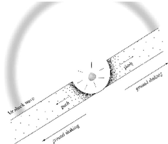
Figure 1. A common schema of main explosion factors influencing on snow stability.
