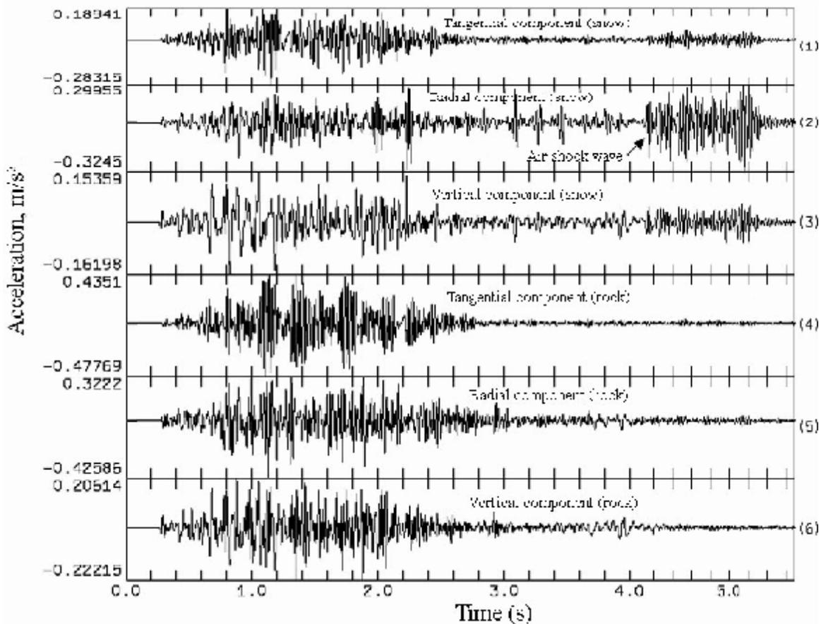
Figure 5. An example of acceleration records for snow surface and underlying surface (rock).
