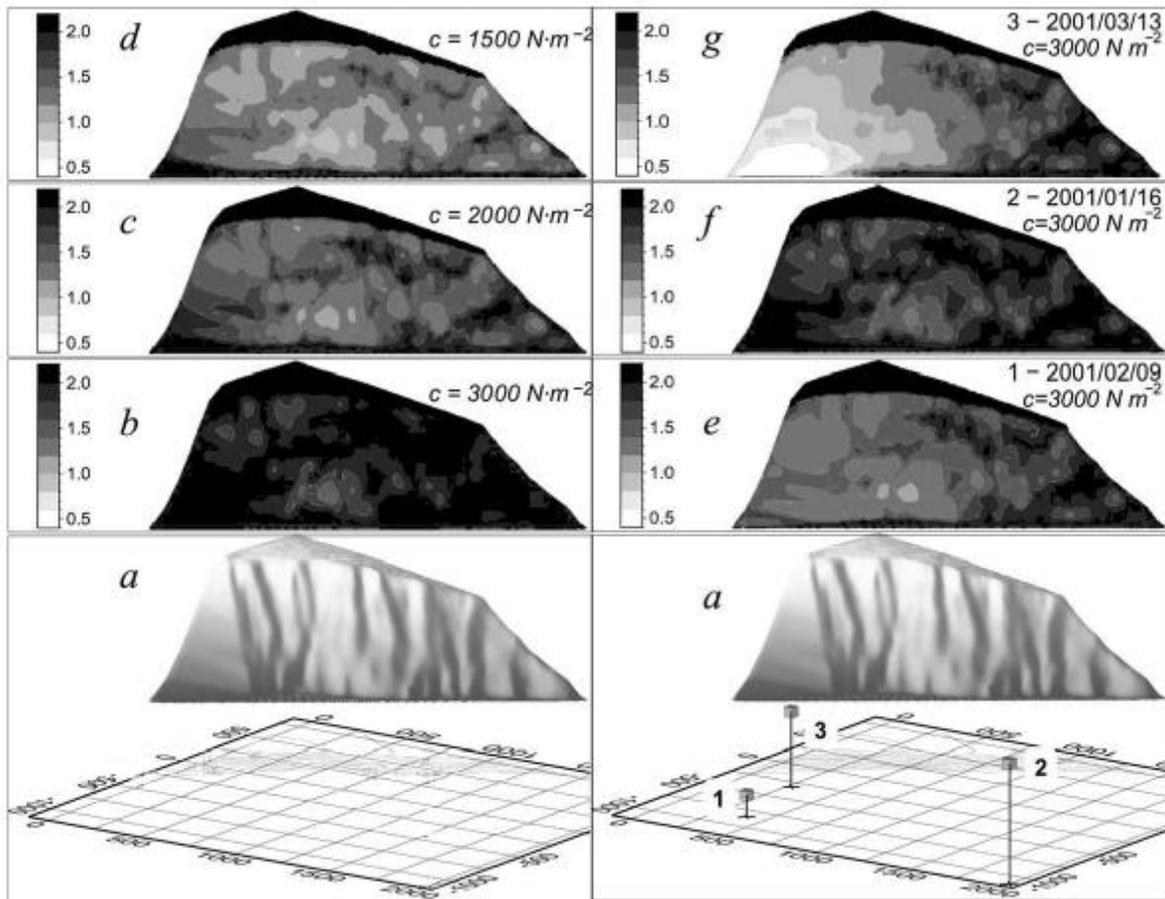
Figure 9. The static probabilistic analysis results. A left-hand panel represents the stability factor distribution with no seismic load while a right-hand panel demonstrates risk changes induced by the explosion dated by 04/06/2001.  $F$  is the stability factor.  $F > 1$  for a stable snow pack and  $F < 1$  – for an unstable snow pack (Chernouss et al., 2002).
