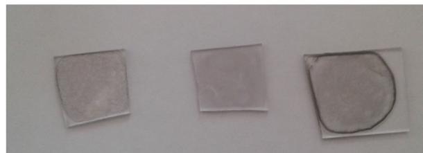
**Figure 5.** SWCNT composites with TRELENA 009, 010, 013 (from left to right).
