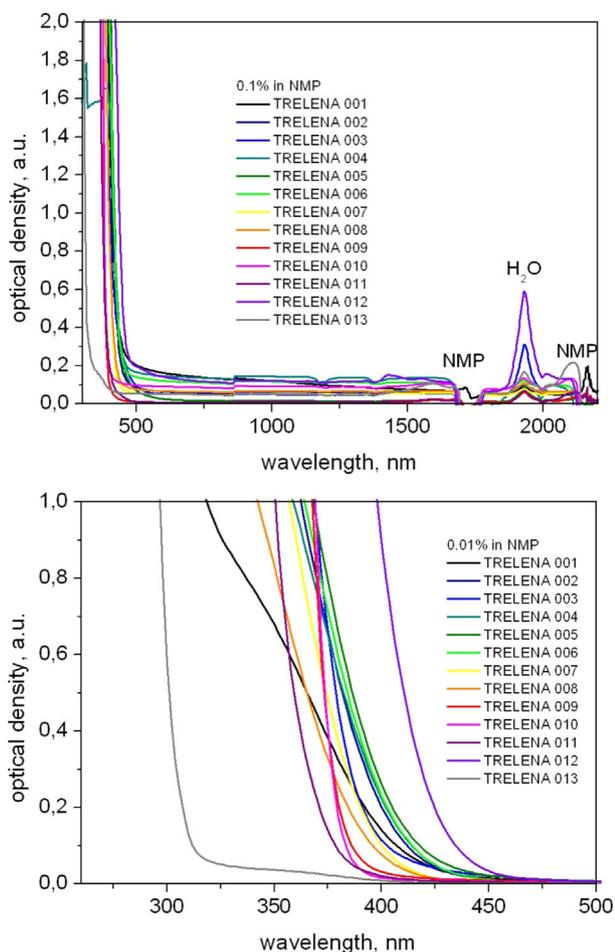
**Figure 2.** Optical absorption spectra of selected polyimides.
