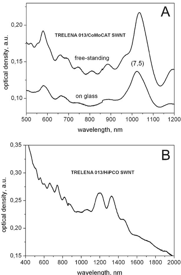
**Figure 6.** The optical absorption spectra of composite films SWCNT/TRELENA 013. A) Films with CoMoCAT nanotubes with small diameters ( $0.7\ \text{nm}$ ). B) Films with HipCO nanotubes (diameters  $0.7\text{--}1.4\ \text{nm}$ ).
