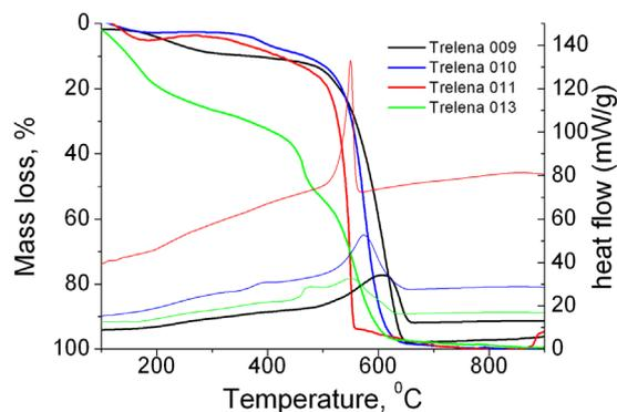
**Figure 3.** Mass loss and heat flow in temperature range 100–900 °C for polyimides TRELENA 009–011, 013.
