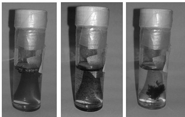
**Figure 4.** Aggregation of nanotubes in polyimide/NMP after the centrifuging at  $150\,000\times g$  right after the centrifuging, after 20 min, and after 1 h.
