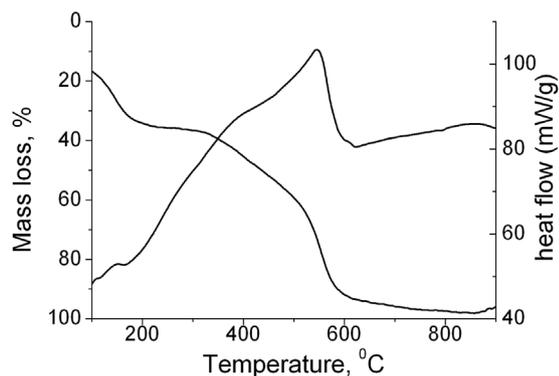
**Figure 7.** Mass loss and heat flow in the temperature range 100–900 °C for composite film SWCNT/TRELENA 013.
